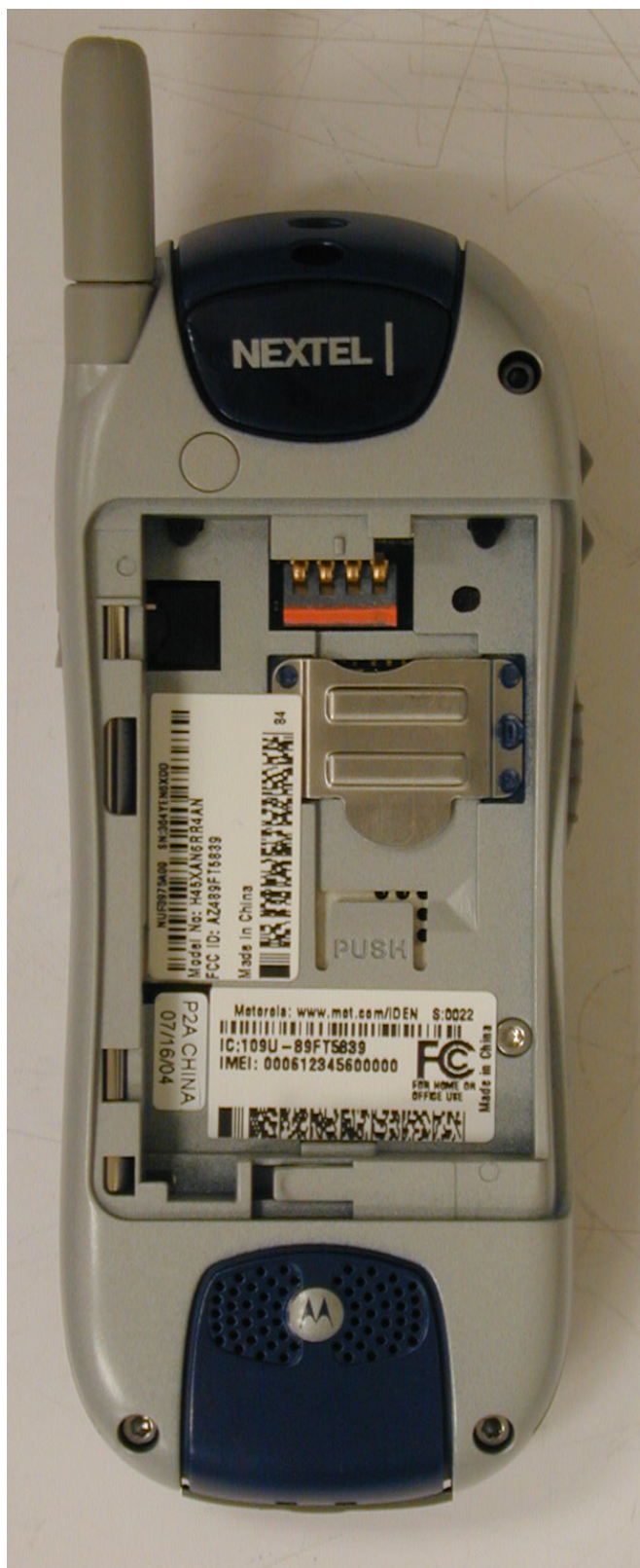
Photograph 3.9: Location of label on back of unit's housing (battery cover removed).
