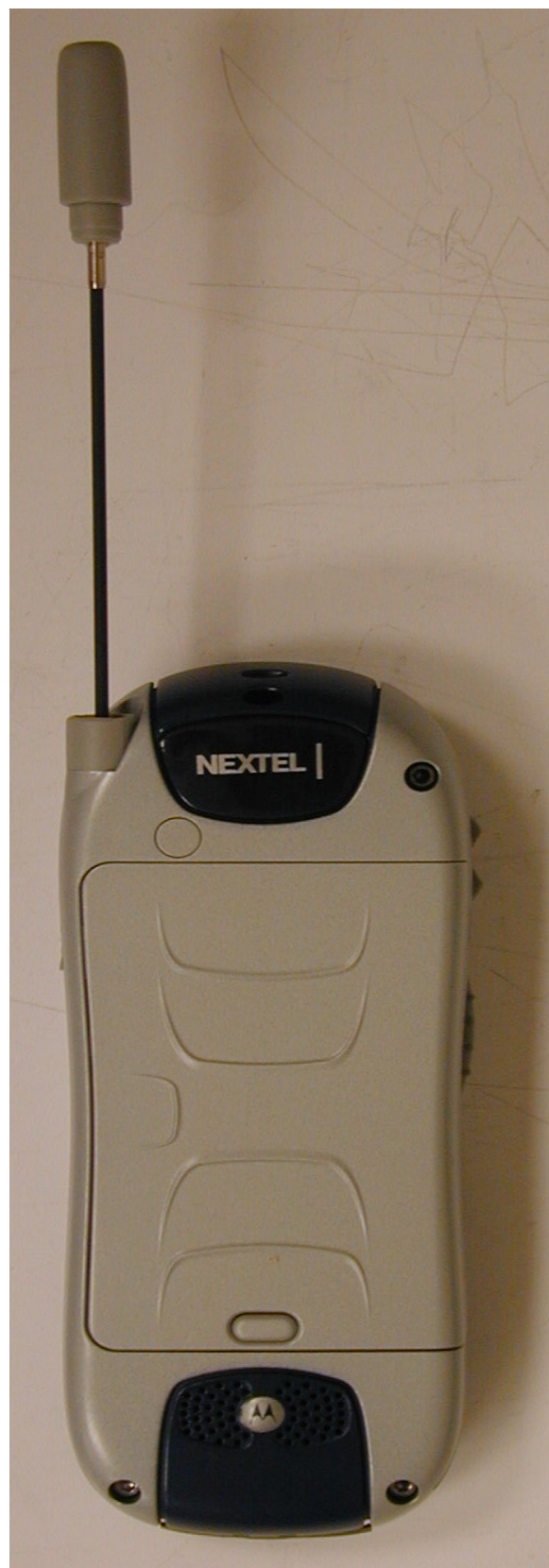
Photograph 3-4: Back view, antenna extended battery cover attached.
