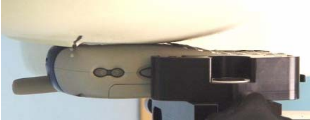
Figure 5. Assessment @ the Right ear DUT in 15° tilt position (same position used for antenna extended)
