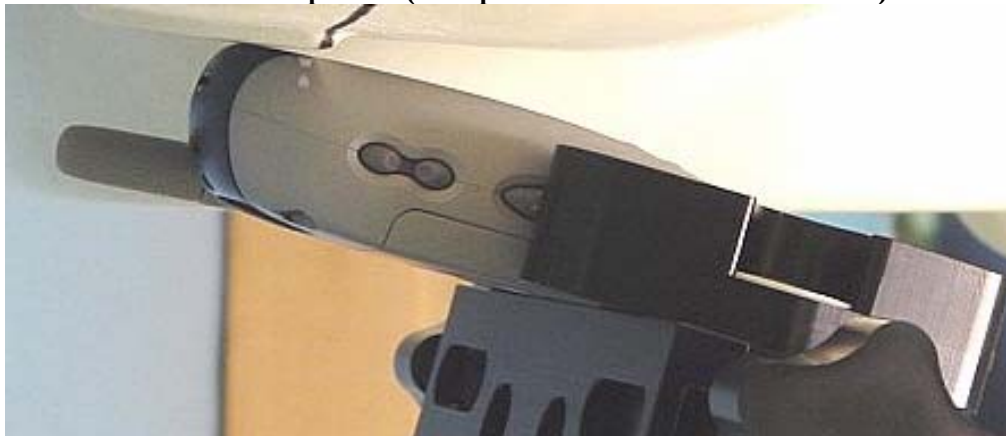
Figure 5. Assessment @ the Right ear DUT in 15° tilt position (same position used for antenna extended)
