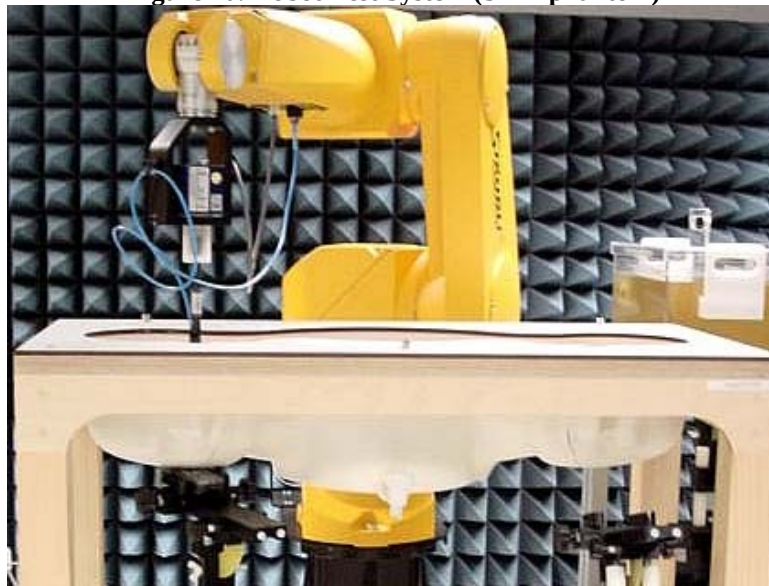
Figure 10: Robot Test System (SAM phantom)
