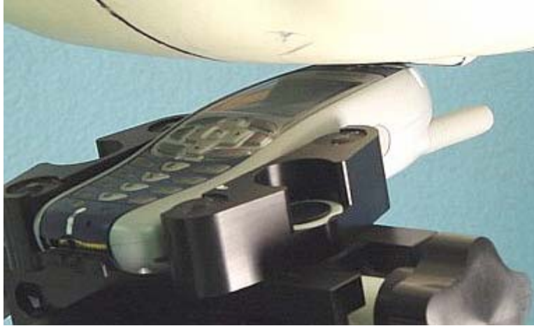
Figure 4. Assessment @ the Right ear DUT in Cheek touch position (same position used for antenna extended)
