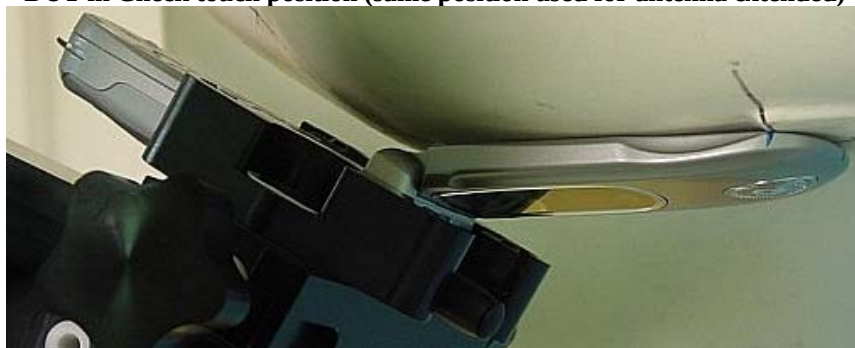
Figure 2. Assessment @ the Left ear DUT in Cheek touch position (same position used for antenna extended)
