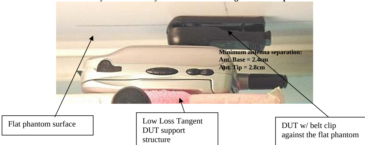
Figure 2. Assessment @ the Left ear DUT in Cheek touch position (same position used for antenna extended)
