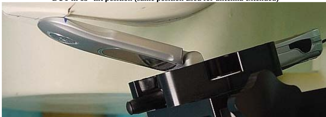
Figure 5. Assessment @ the Right ear DUT in 15° tilt position (same position used for antenna extended)
