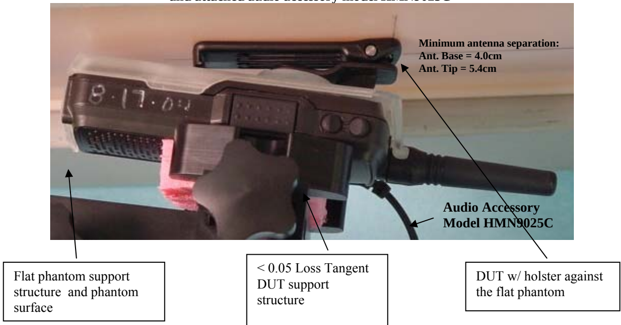
Figure 2: Highest S.A.R. Test Position (@ body) DUT with body worn accessory model RLN5713A against the flat phantom and attached audio accessory model HMN9025C
