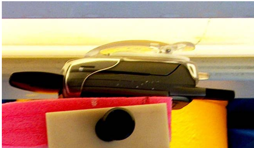
Figure 2: Highest S.A.R. Test Position (Body) DUT with carry accessory model NNTN6026A against the phantom.
