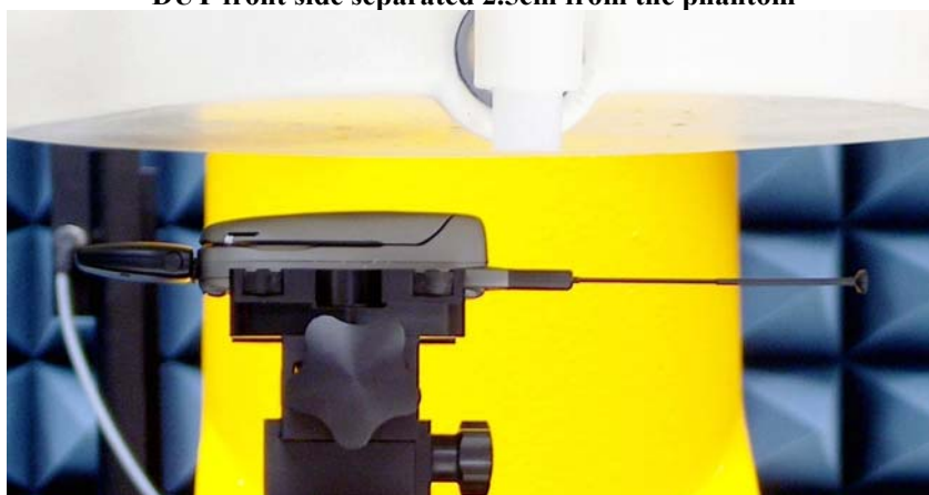
Figure 5: Highest S.A.R. Test Position (face) DUT front side separated 2.5cm from the phantom
