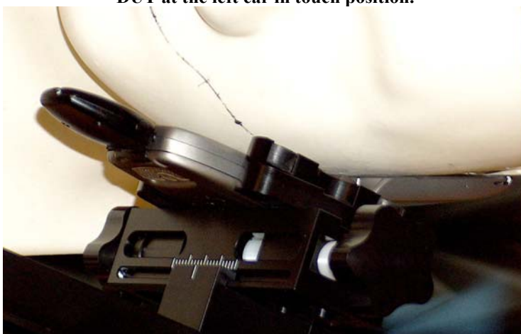
Figure 5: Highest S.A.R. Test Position (face) DUT front side separated 2.5cm from the phantom
