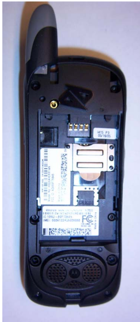
Photograph 1.1: Location of label on back of unit's housing (battery cover removed).
