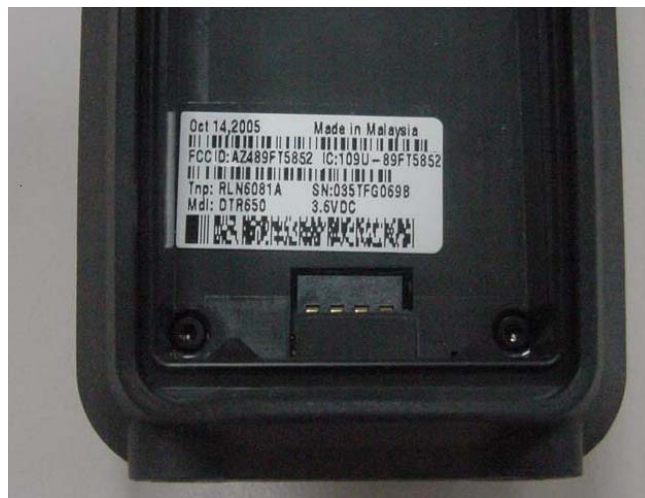
Figure 1-1: Location of the FCC label in the radio
