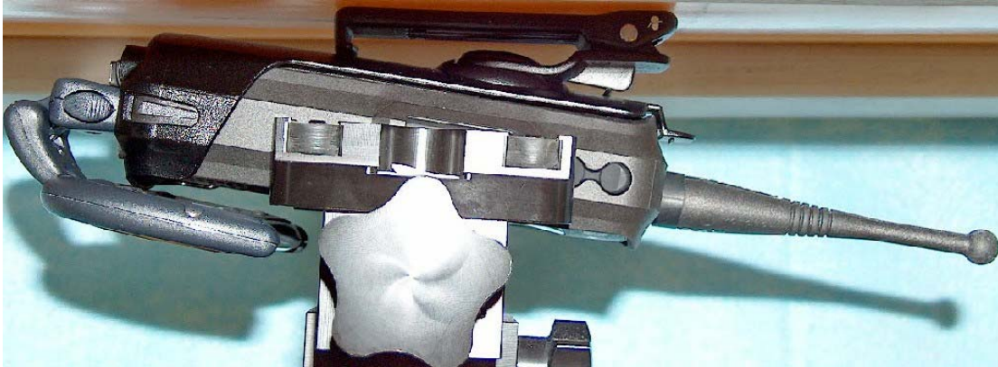
Figure 1: Highest S.A.R. Test Position (Body) DUT with body worn accessory model RLN5713A and attached data accessory model NNTN5491A (Same position used for all other attached accessories at the body)
