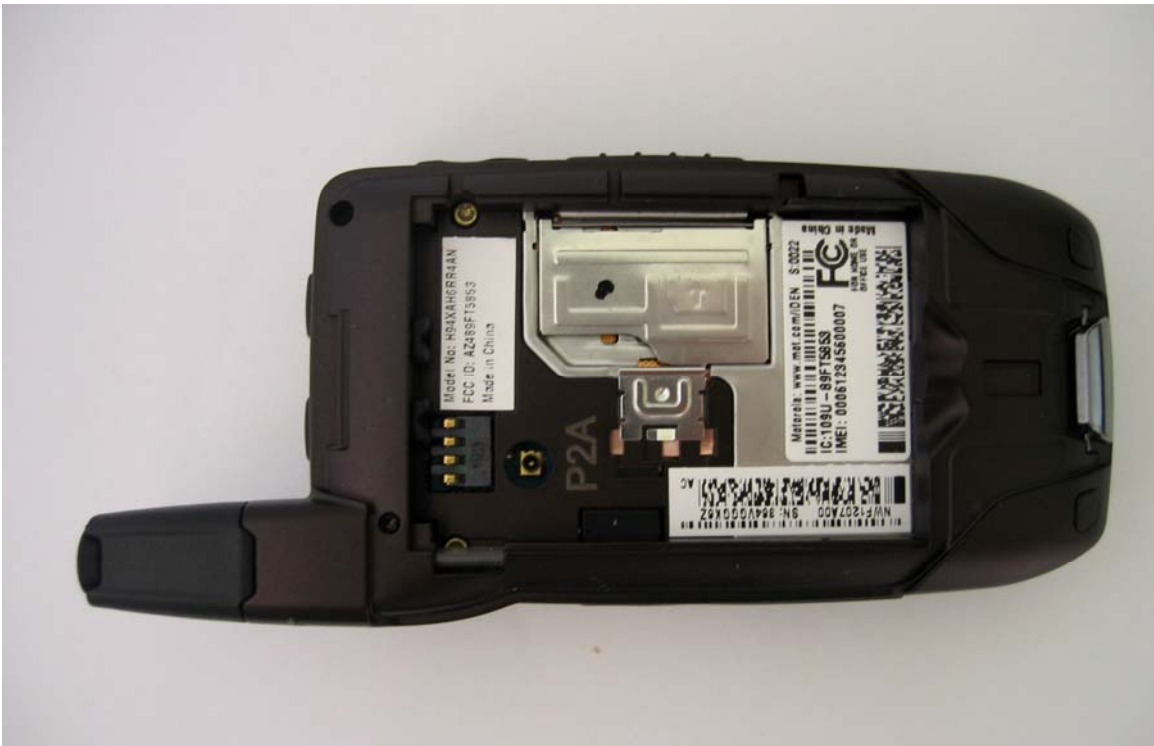
Figure 3-14. Battery Compartment of i880 radio.
