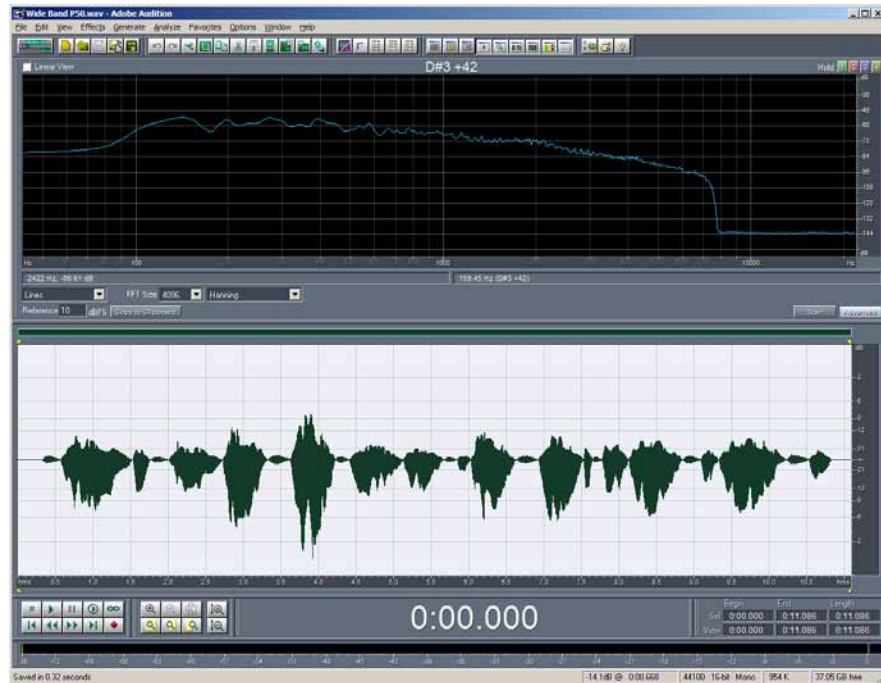
Figure 6.4.1-1 Wide Band P50 Frequency Response and Time Domain Hanning Windowing Function and 4026 FFT Size
