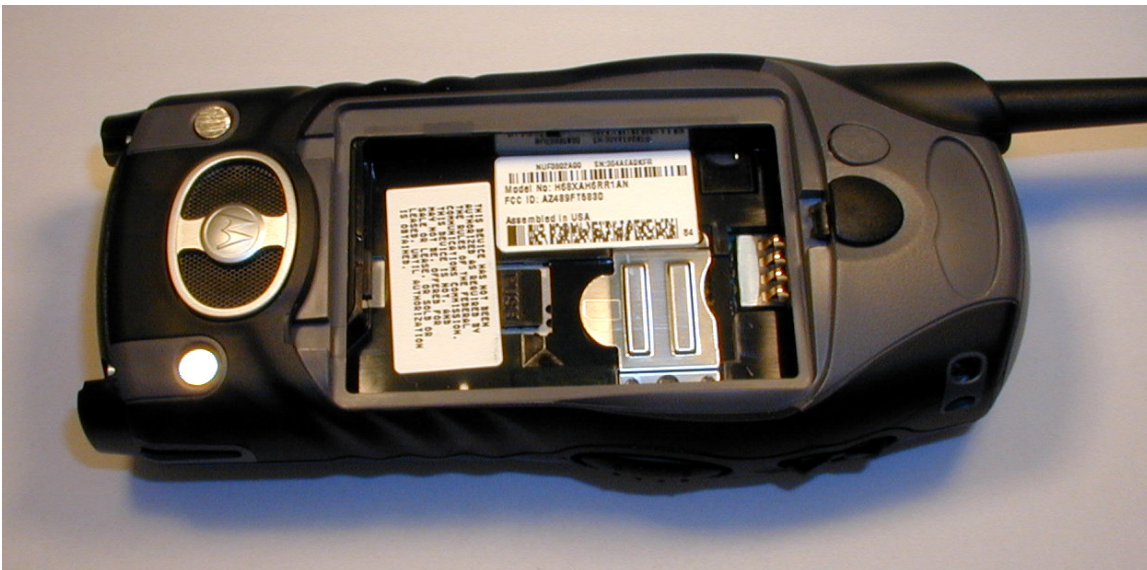
Photograph 1.1: Back of radio battery compartment, showing label locations.
