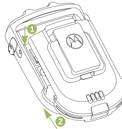
Figure 2.2: Attaching the battery into the WRSM
