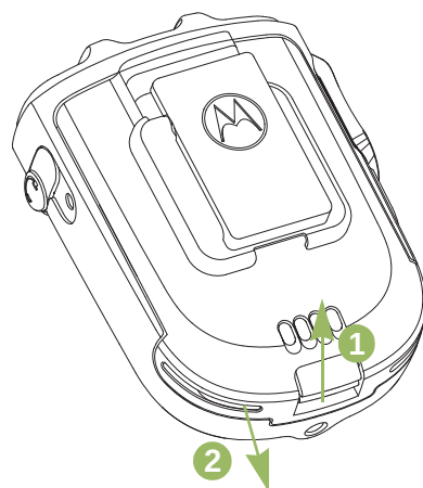
Figure 2.3: Removing the battery from the WRS
