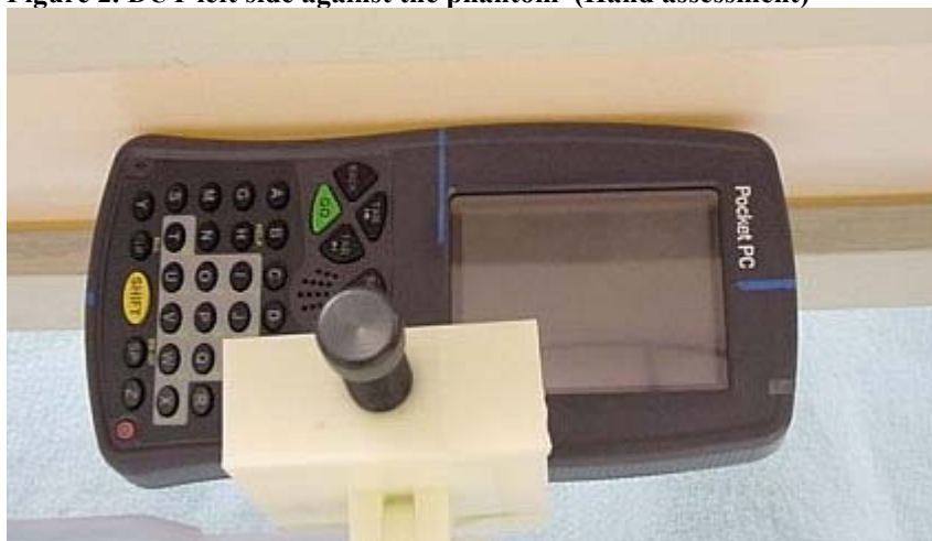
Figure 2. DUT left side against the phantom (Hand assessment)
