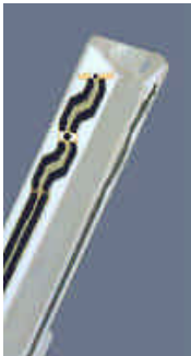
Figure 3.2 Probe Thick-Film Technique
