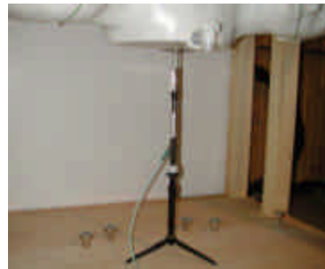
Figure 12.1 Dipole Validation Test Setup
