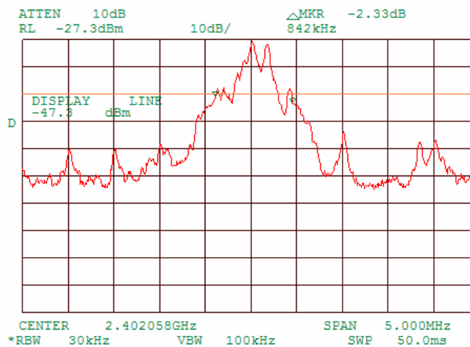
Plot 8.2.1 20 dB bandwidth test result at low frequency, 1 MBPS
