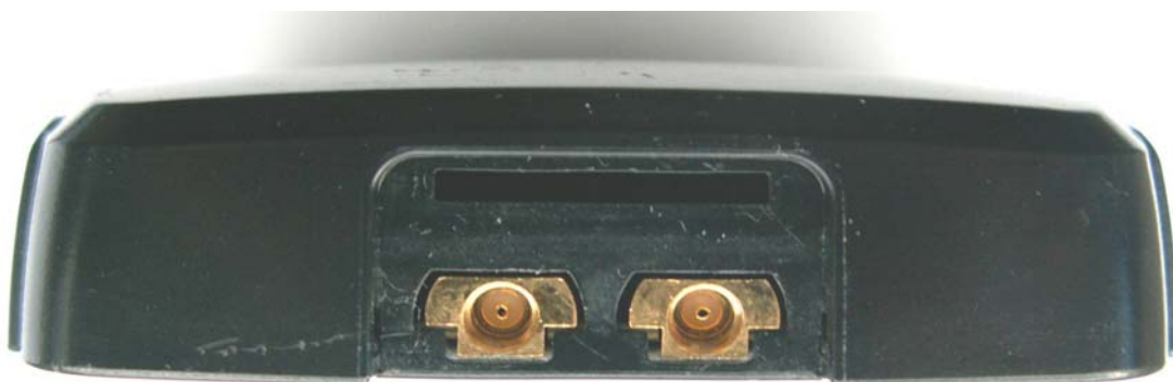
Photograph 3.4: Front view of WDE1000 – External RF connectors.
