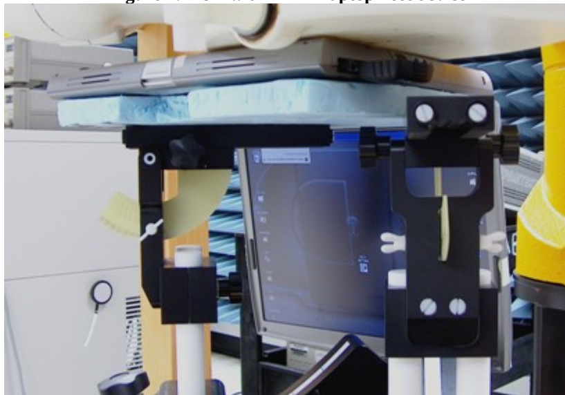
Figure 2: DUT with DELL laptop host device
