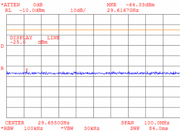
Plot 6.6.46: Tx Conducted spurious emission measurements at the 6 th harmonic of low carrier frequency, OBW 5 MHz
