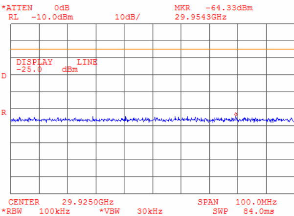
Plot 6.6.48: Tx Conducted spurious emission measurements at the 6 th harmonic of high carrier frequency, OBW 5 MHz
