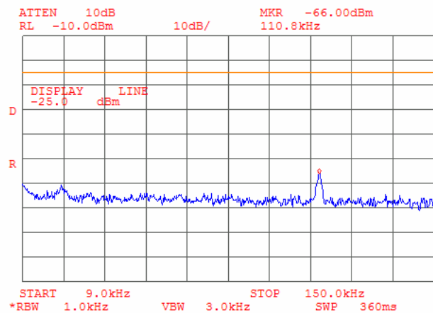
Plot 6.6.1: Tx Spurious emission measurements in 9 - 150 KHz range at low carrier frequency, OBW 5 MHz
