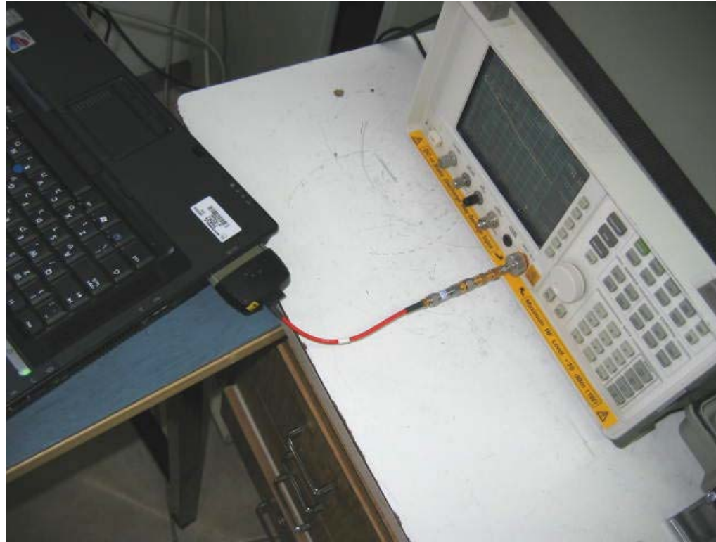
Photograph 7.4: Conducted spurious emission Measurements setup for 802.11a @ 4.9GHz
