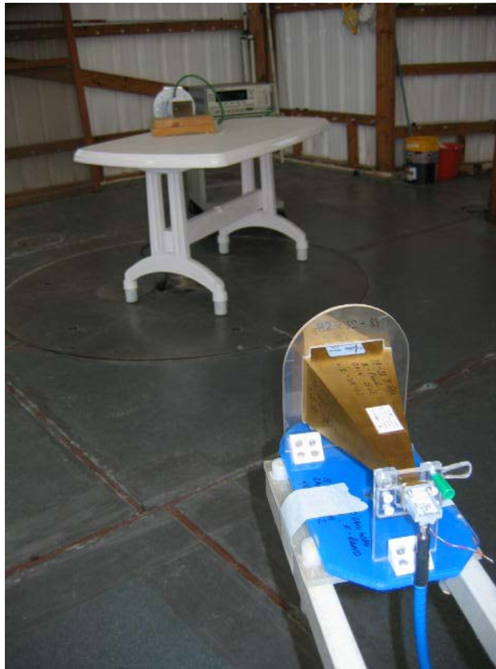
Photograph 7.12: Substitution ERP measurements setup from 18 to 26.50 GHz at OATS
