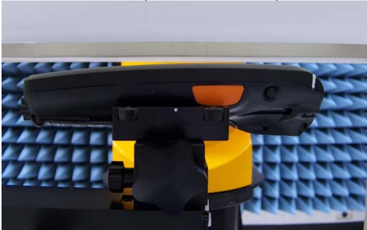
Figure 4: Highest S.A.R. Test Position (Face) DUT front side separated 2.5cm from the phantom
