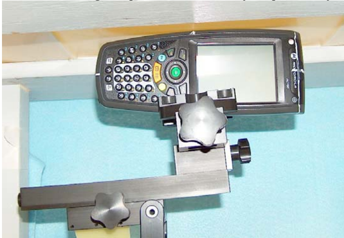
Figure 6: Hand Assessment DUT left side against phantom without carry strap accessory
