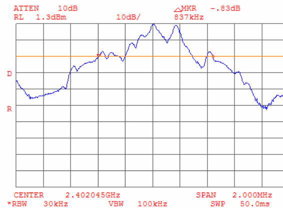
Plot 8.2.2 The 20 dB bandwidth test result at mid frequency
