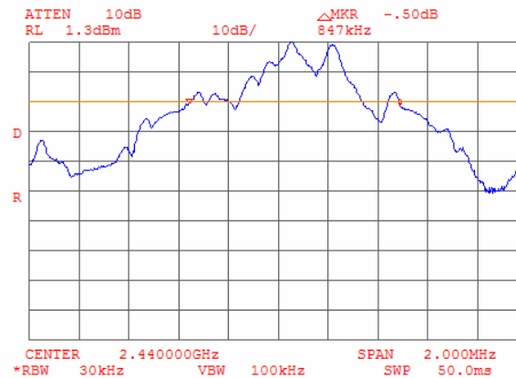
Plot 8.2.2 The 20 dB bandwidth test result at mid frequency
