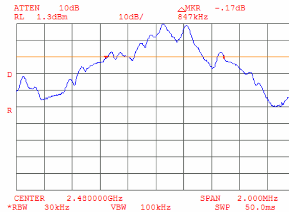
Plot 8.2.3 The 20 dB bandwidth test result at high frequency
