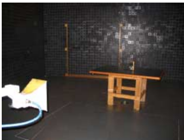
Photograph 8.1.3 Setup for spurious emission field strength measurements above 1000 MHz at anechoic chamber
