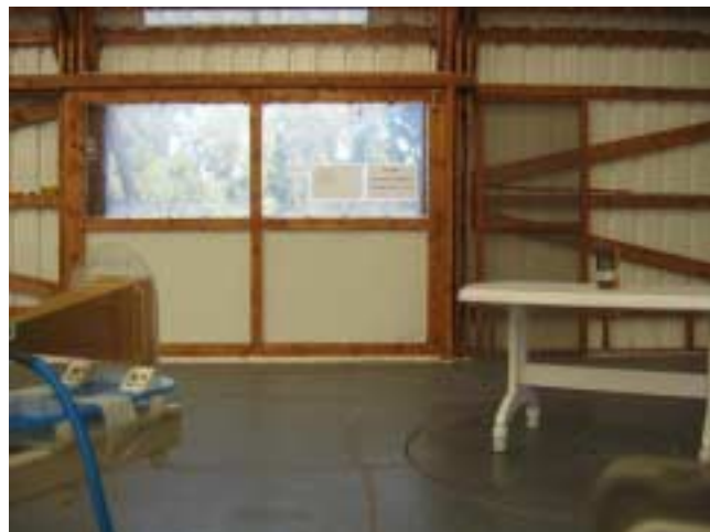
Photograph 8.1.5 Setup for spurious emission field strength measurements above 18 GHz at the OATS
