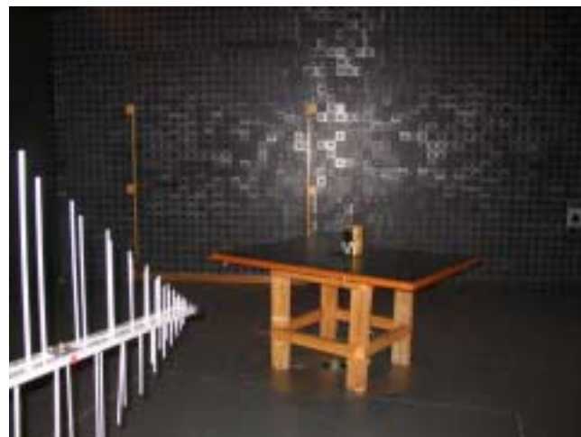
Photograph 8.1.2 Setup for spurious emission field strength measurements from 30 to 1000 MHz
