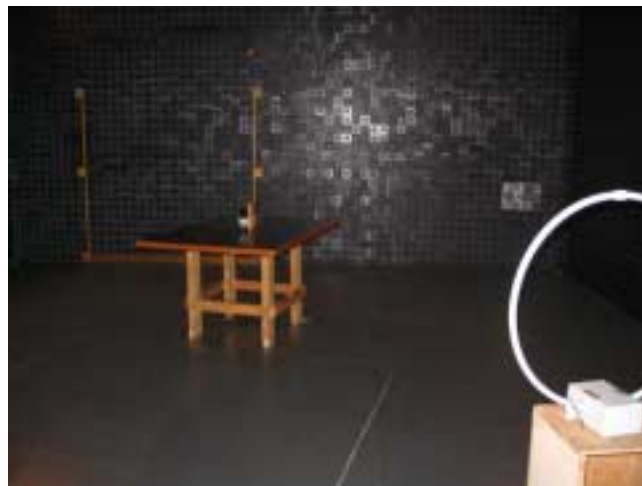
Photograph 8.1.1 Setup for spurious emission field strength measurements below 30 MHz
