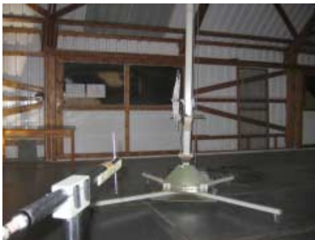
Photograph 7.1.2 Setup for substitution peak output power measurements
