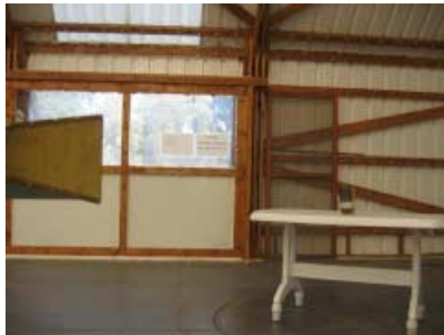
Photograph 8.1.5 Setup for spurious emission field strength measurements above 18 GHz at the OATS
