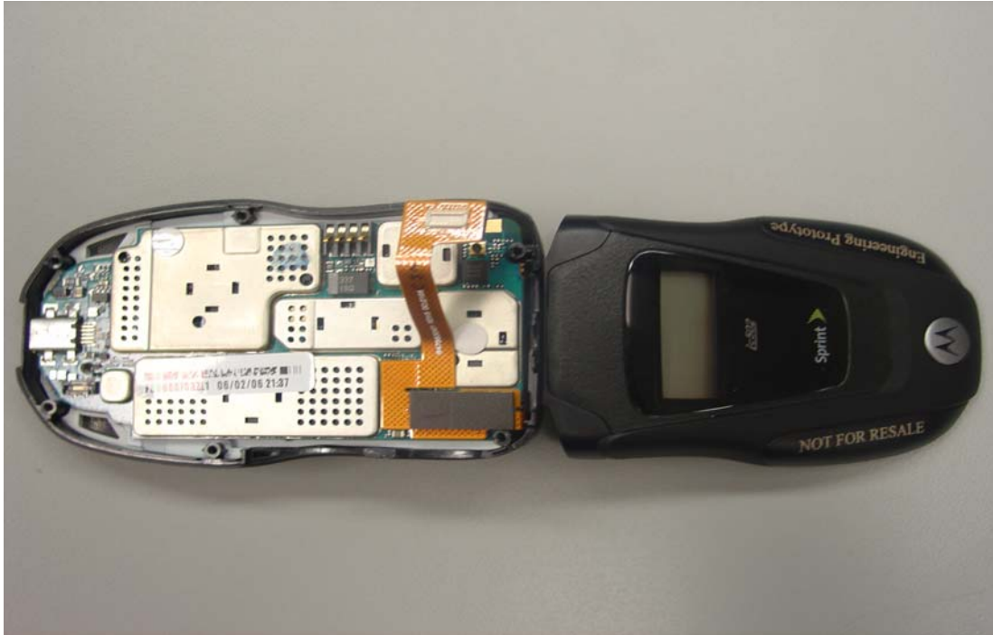
Photograph 9-1: Back side view of radio product PC Board
