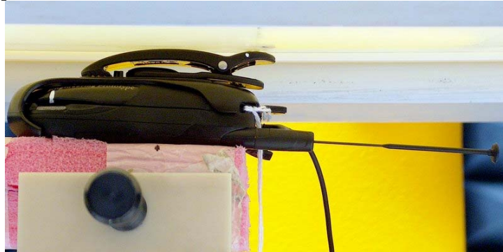
Figure 1: Highest S.A.R. Test Position (Body) DUT w/ holster against the phantom; worst case audio accessory attached, and antenna extended (same position used for all other audio/data accessories and for ant retracted)
