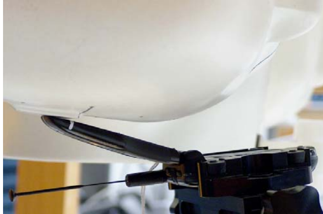
Figure 7: Assessment at the Head DUT at the right ear in tilt position. (same position used for antenna retracted)
