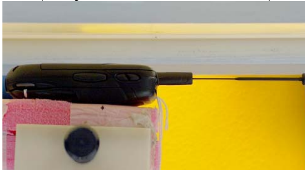
Figure 4: Body Assessment DUT w/ back side separated 2.5cm from the phantom. (same position used for antenna retracted)
