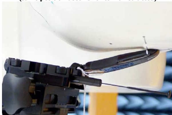
Figure 9: Assessment at the Head DUT at the left ear in tilt position. (same position used for antenna retracted)
