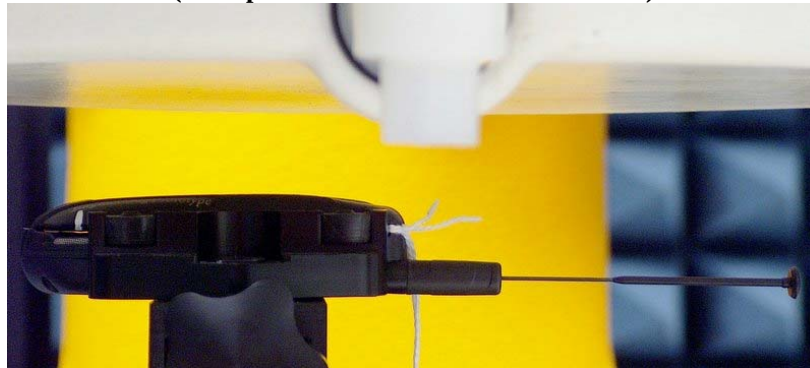
Figure 2: Highest S.A.R. Test Position (face) DUT flip closed w/ front side separated 2.5cm from the phantom (same position used for antenna retracted)
