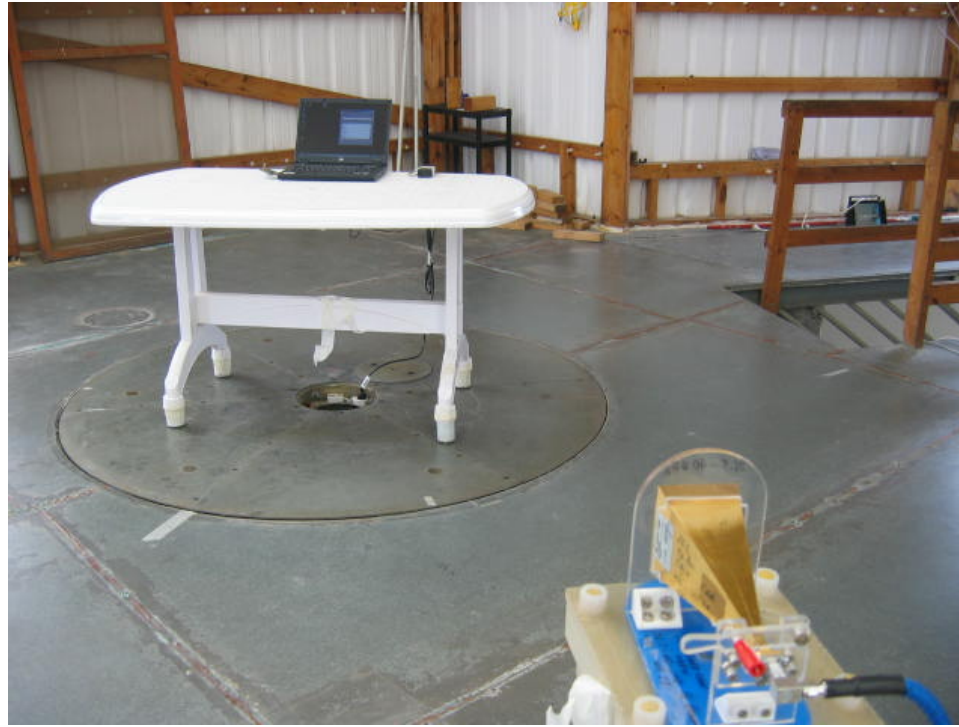
Photograph 7.7: Radiated spurious emission field strength measurements setup at OATS
