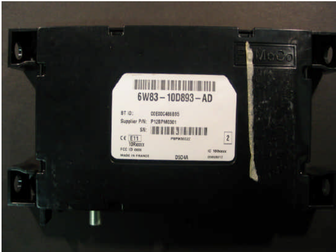
Photo 2: EUT for conducted measurements with temporary antenna connector
