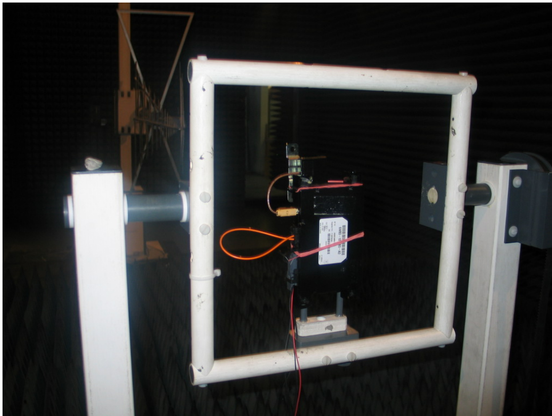
Photo 1: Test setup for radiated measurements.
