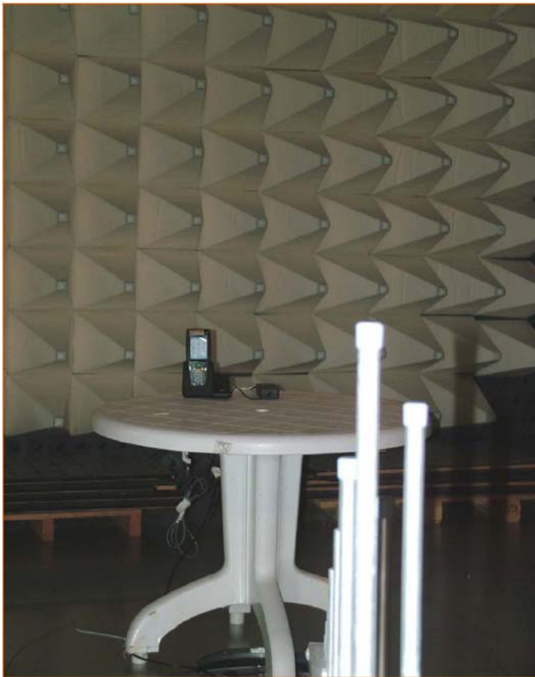
Photograph 5: HC700L Terminal docking into Cradle configuration Radiated Emission Testing
