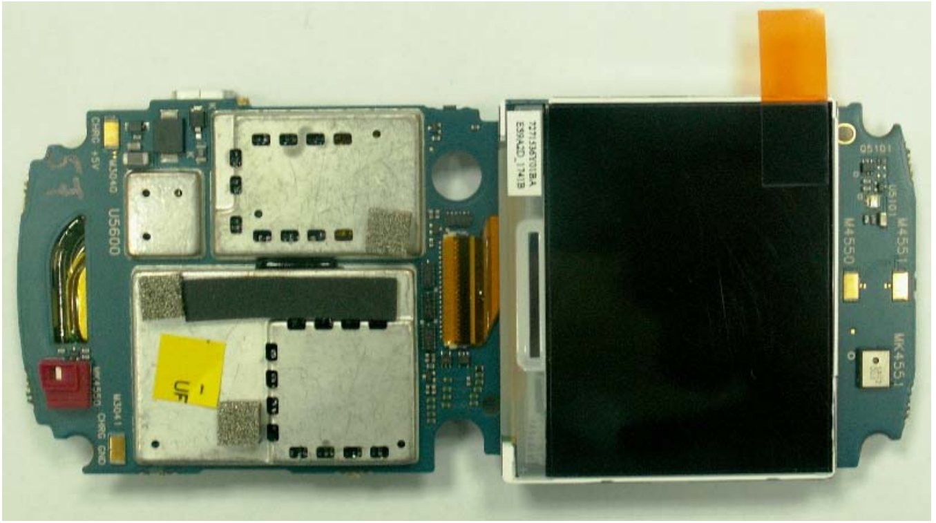
Photograph No. 1 - EWP3100 - Top Side with Shields
