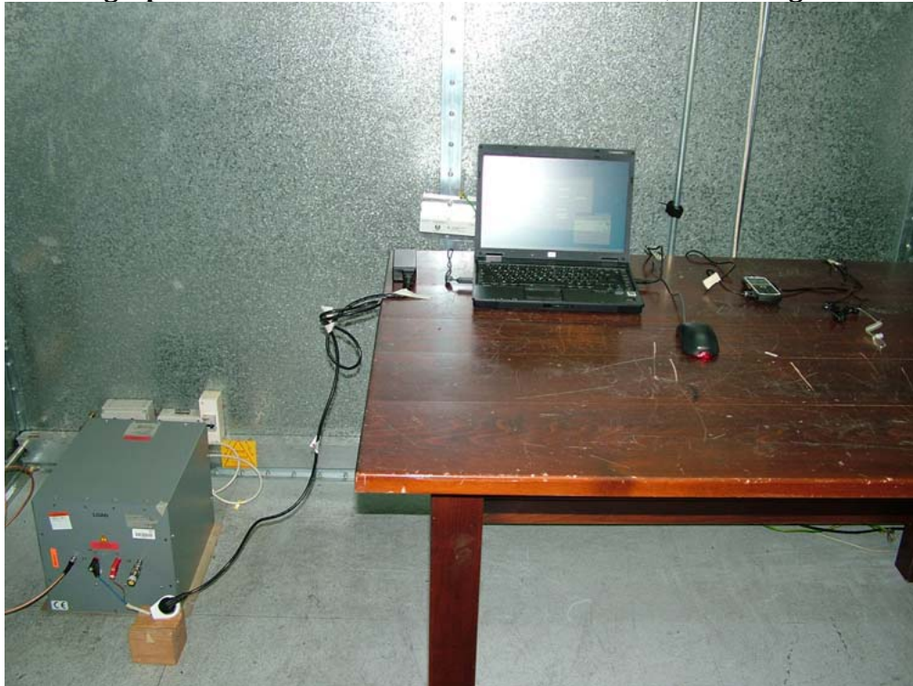
Photograph 3: Power Line Emissions measurement, PC configuration
