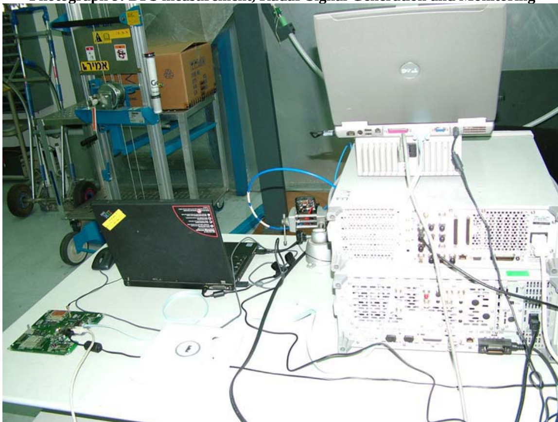
Photograph 9: DFS measurement, Radar Signal Generation and Monitoring
