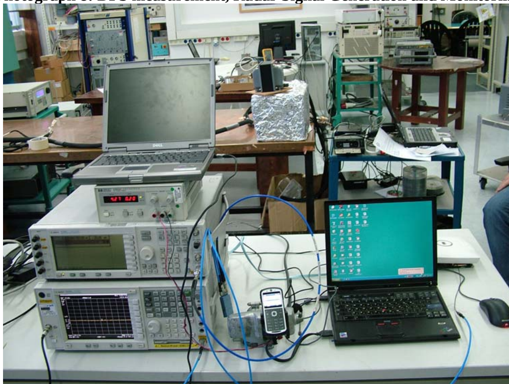
Photograph 8: DFS measurement, Radar Signal Generation and Monitoring,
