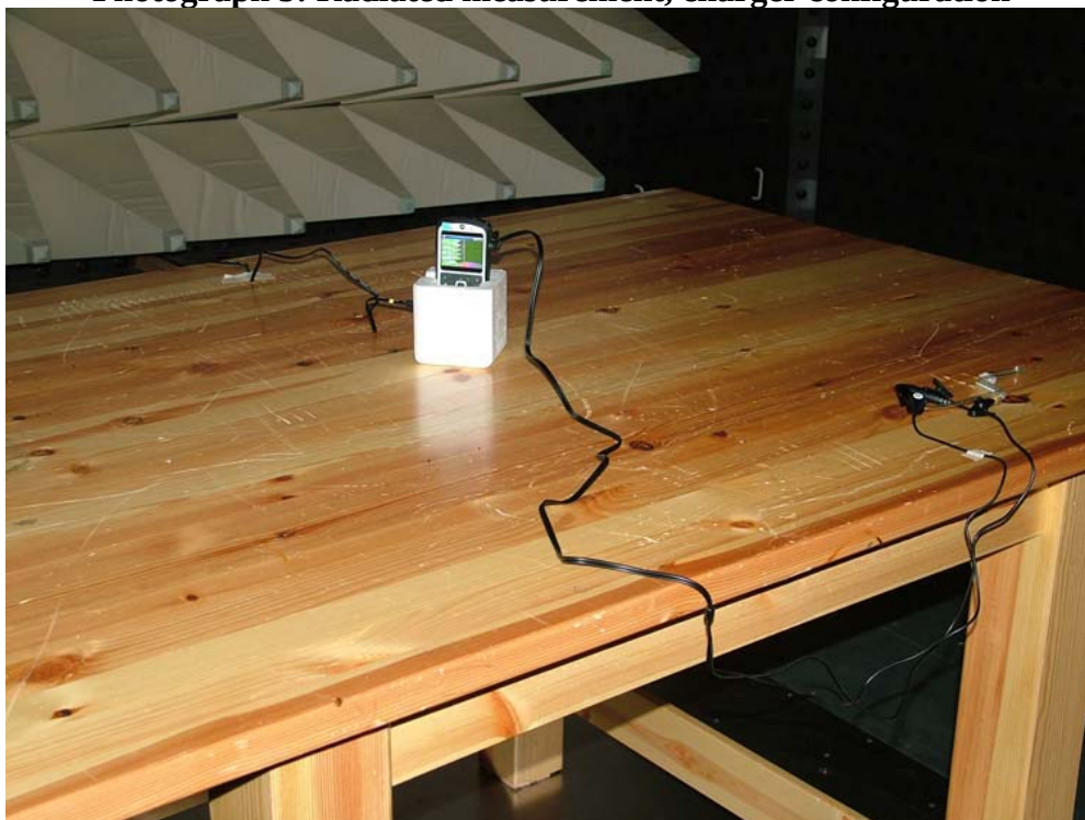
Photograph 5: Radiated measurement, charger configuration
