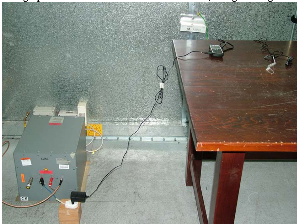
Photograph 2: Power Line Emissions measurement, charger configuration
