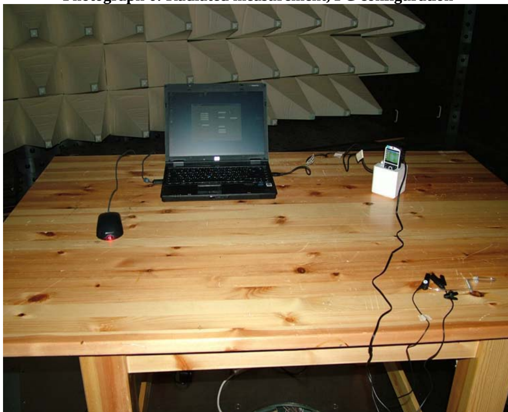
Photograph 6: Radiated measurement, PC configuration
