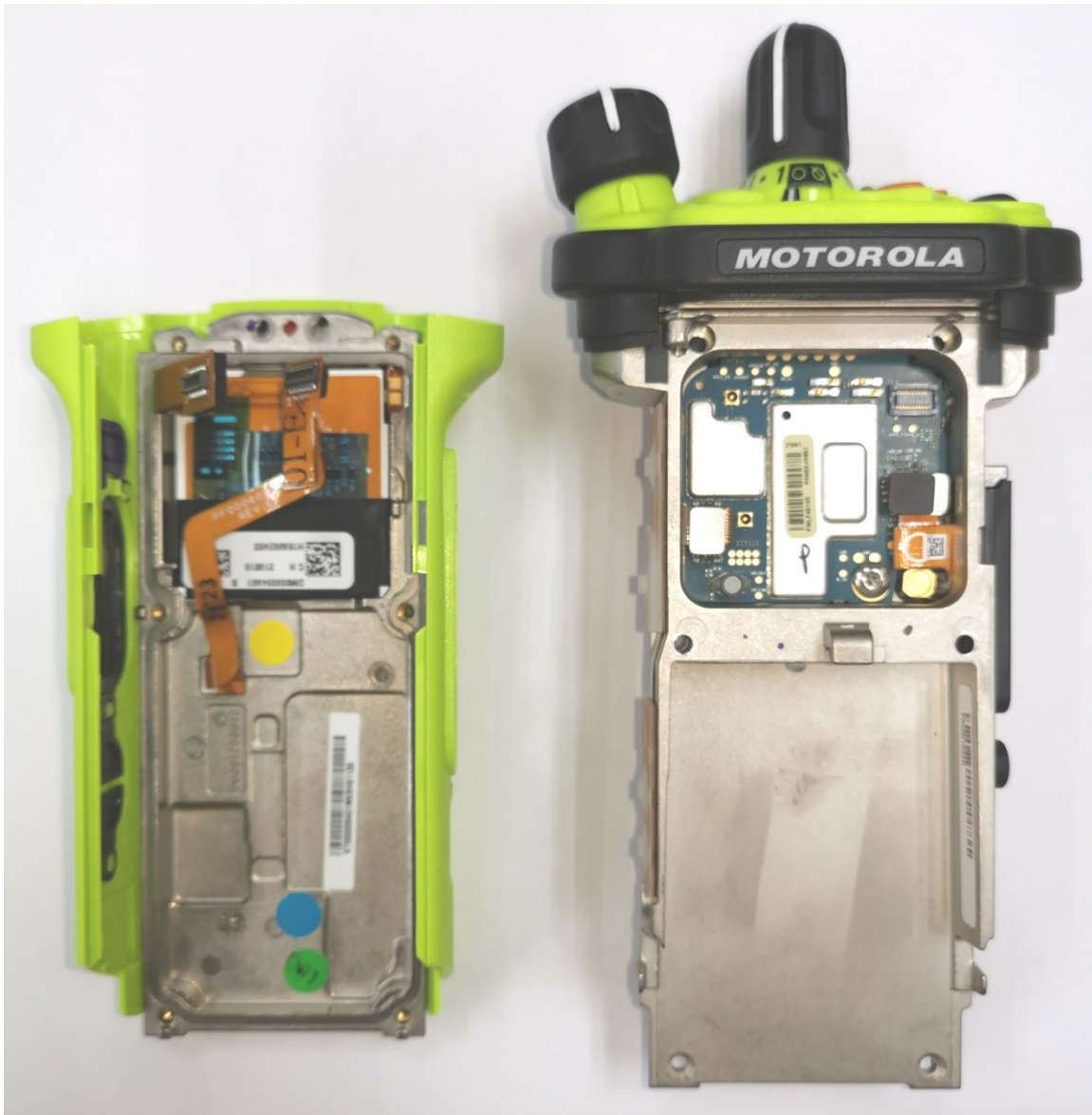
Expansion board with chassis and housing (APX8000XE Model 3.5) (Back Side)
