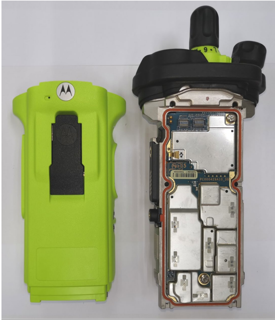
RF and Vocon boards with chassis and housing (APX8000XE Model 1.5) (Front Side)
