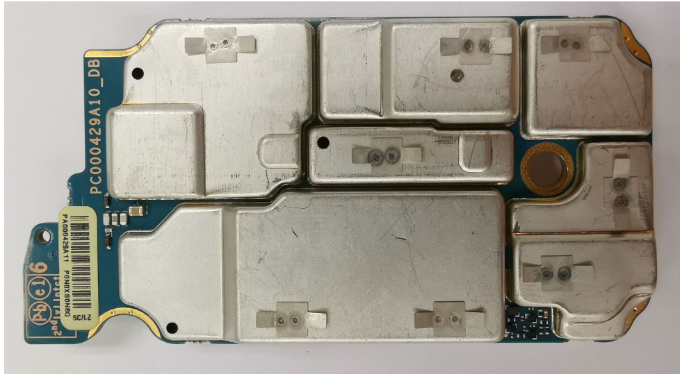
RF board with Shields (Bottom) (APX8000/APX8000XE)
