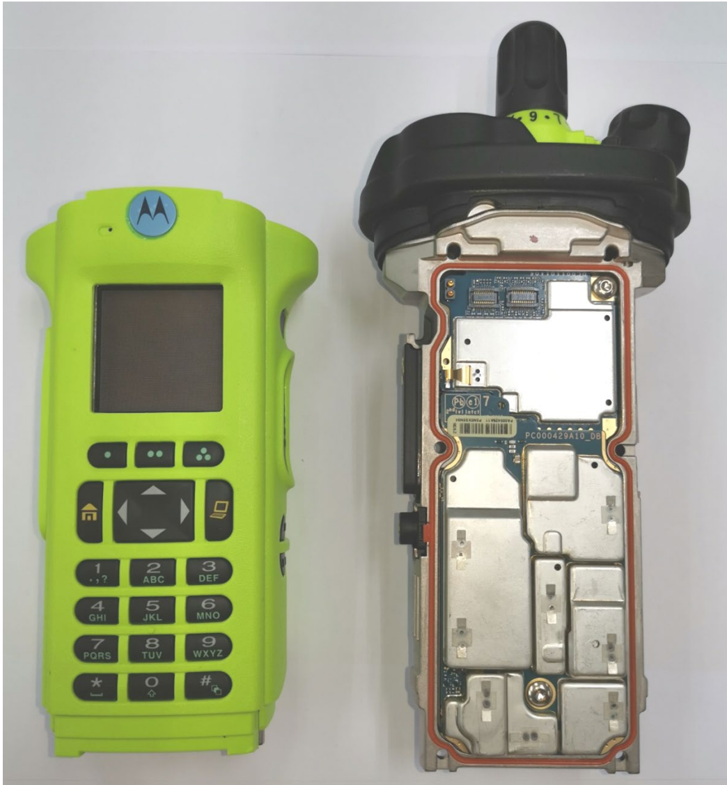
RF and Vocon boards with chassis and housing (APX8000XE Model 3.5) (Front Side)
