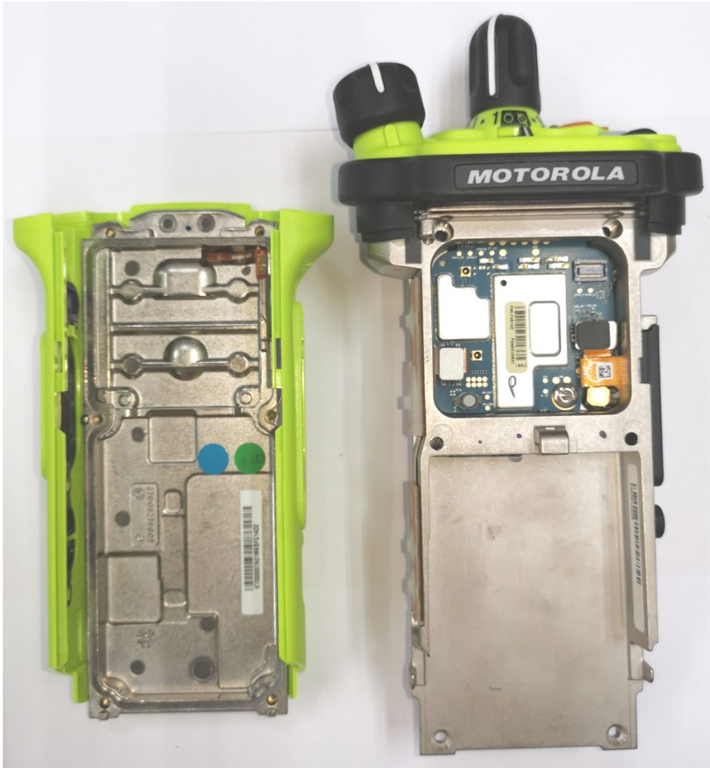
Expansion board with chassis and housing (APX8000XE Model 1.5) (Back Side)
