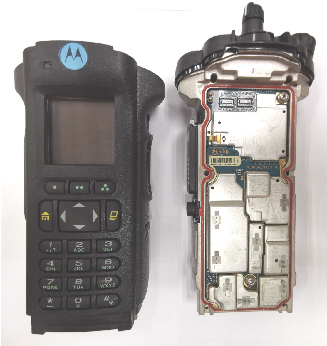
RF and Vocon boards with chassis and housing (APX8000 Model 3.5) (Front Side)
