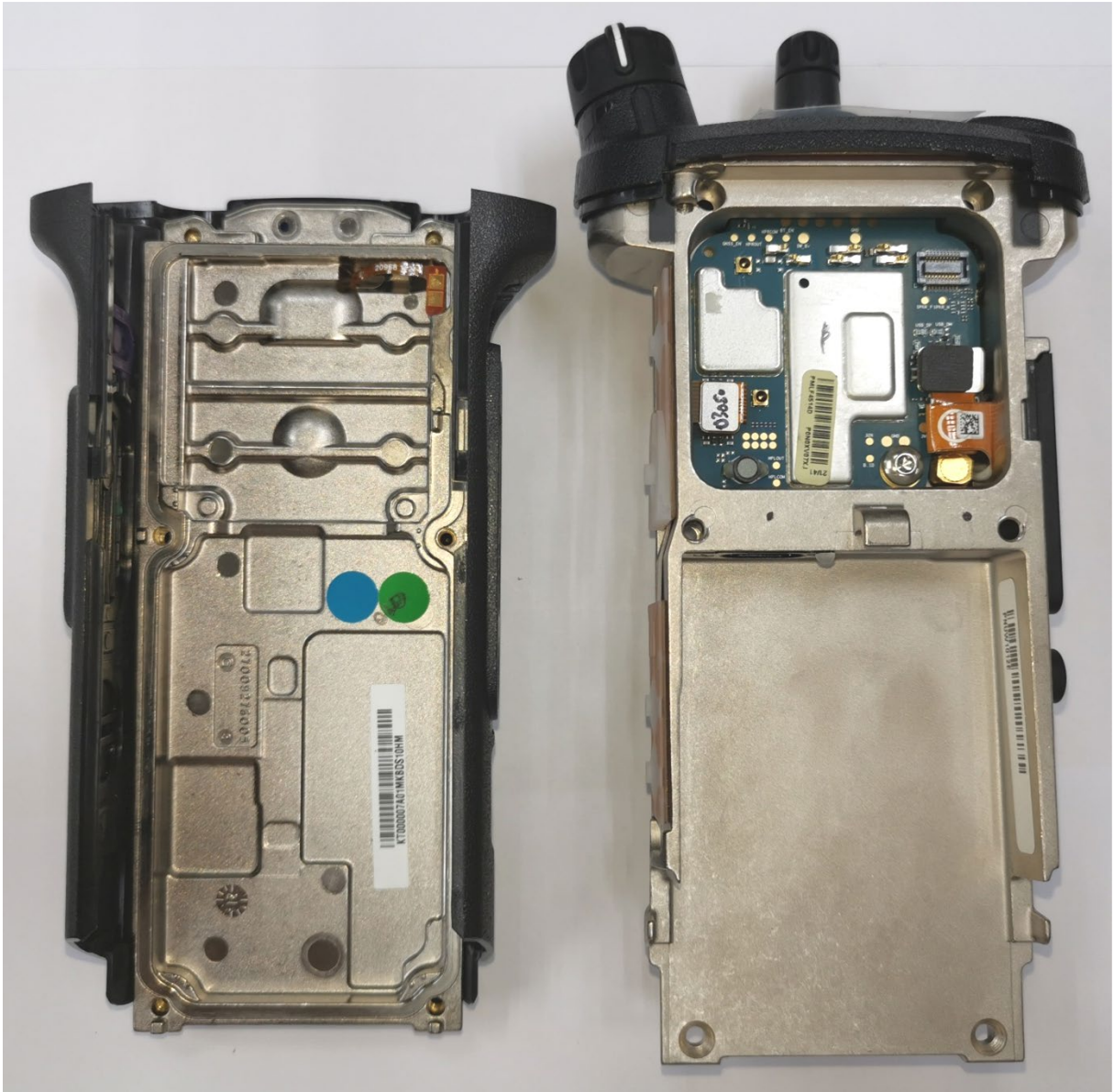
Expansion board with chassis and housing (APX8000 Model 1.5) (Back Side)
