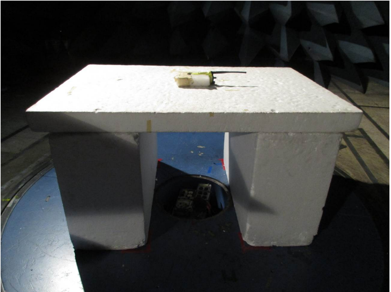
Figure 1: Radiated Emissions – Front View – EUT on Side (Below 1 GHz)
