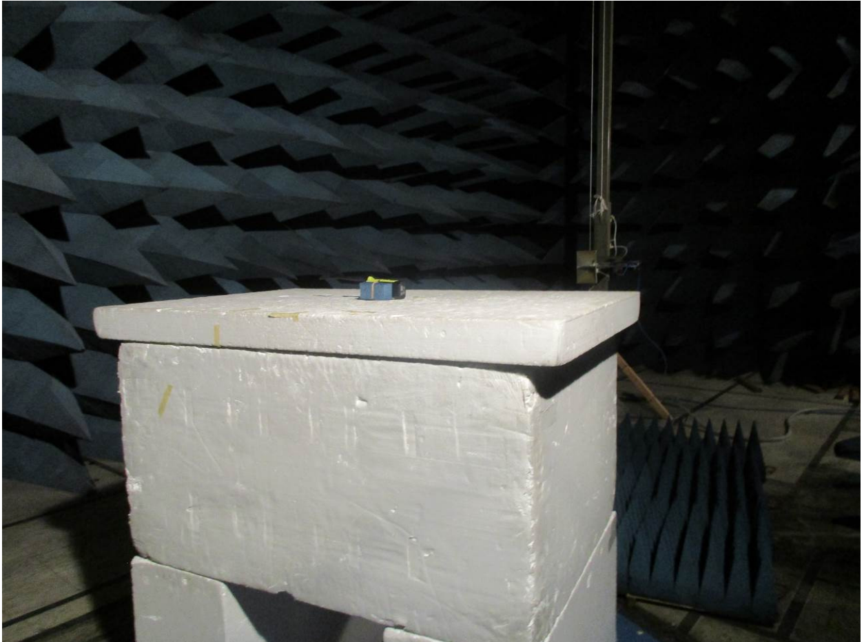
Figure 6: Radiated Emissions – Back View – EUT on Side (Above 1 GHz)
