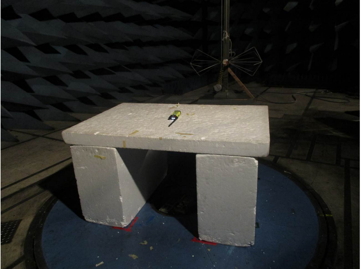
Figure 9: Radiated Emissions – Back View – EUT Flat (30 MHz– 200 MHz)
