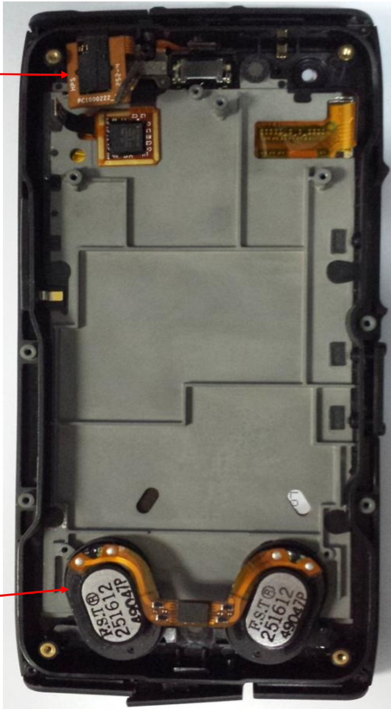
Photograph 9-12: Front housing assembly
