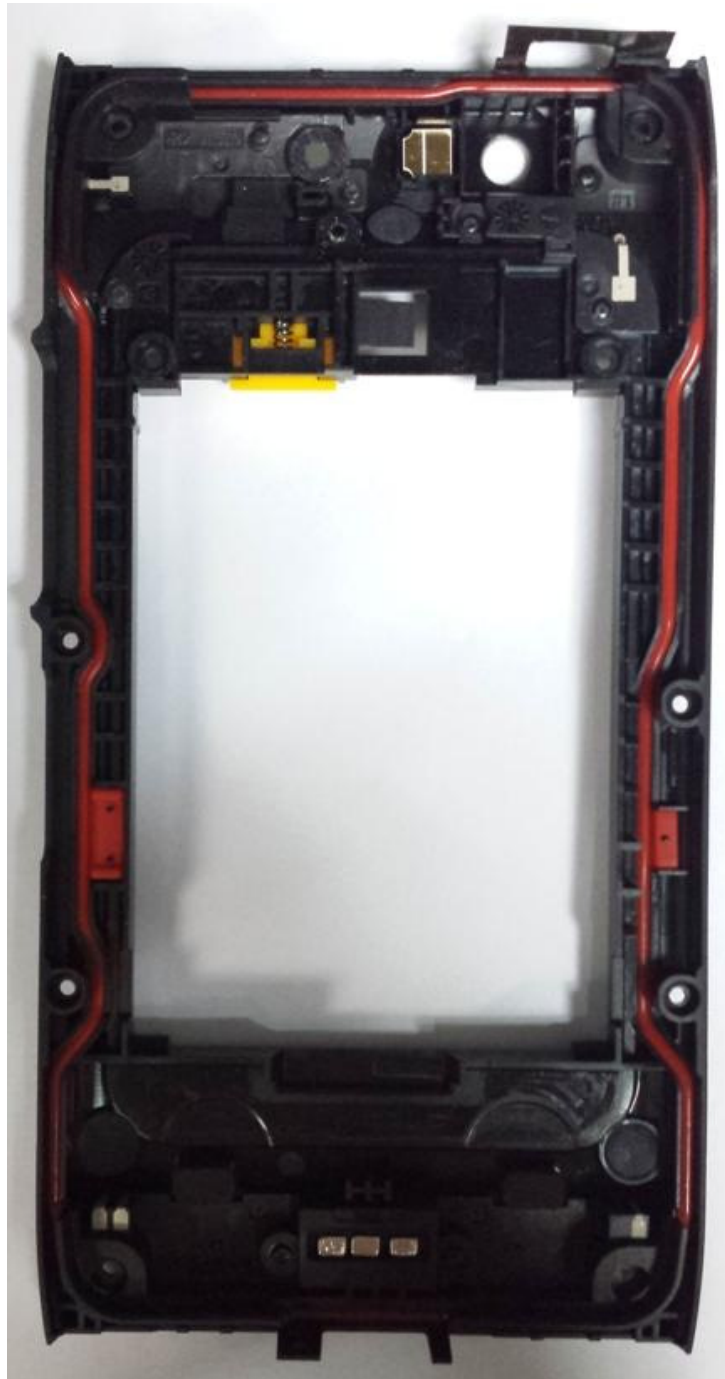
Photograph 9-14: Rear housing assembly
