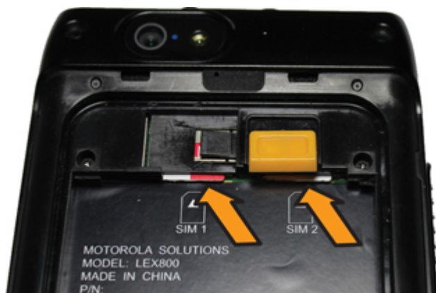
Figure 6: Installing the Public and Private SIM Cards
