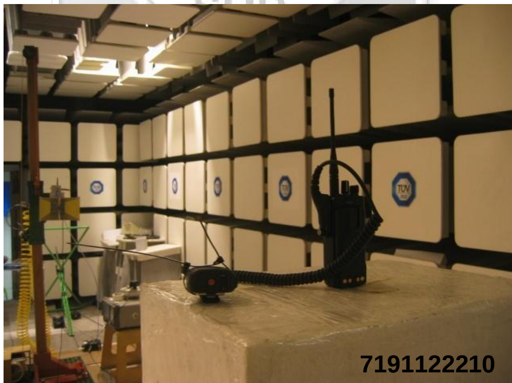
Transmitter Spurious Emissions (Radiated) Test Setup (Rear View)
