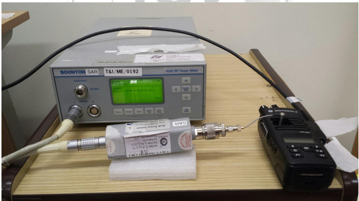
Maximum Peak Power Test Setup
