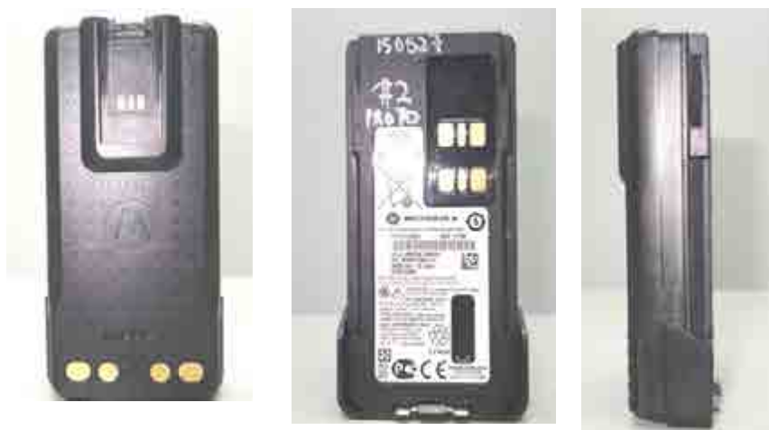
PMNN4488A battery with vibrator (back, front, side view)
