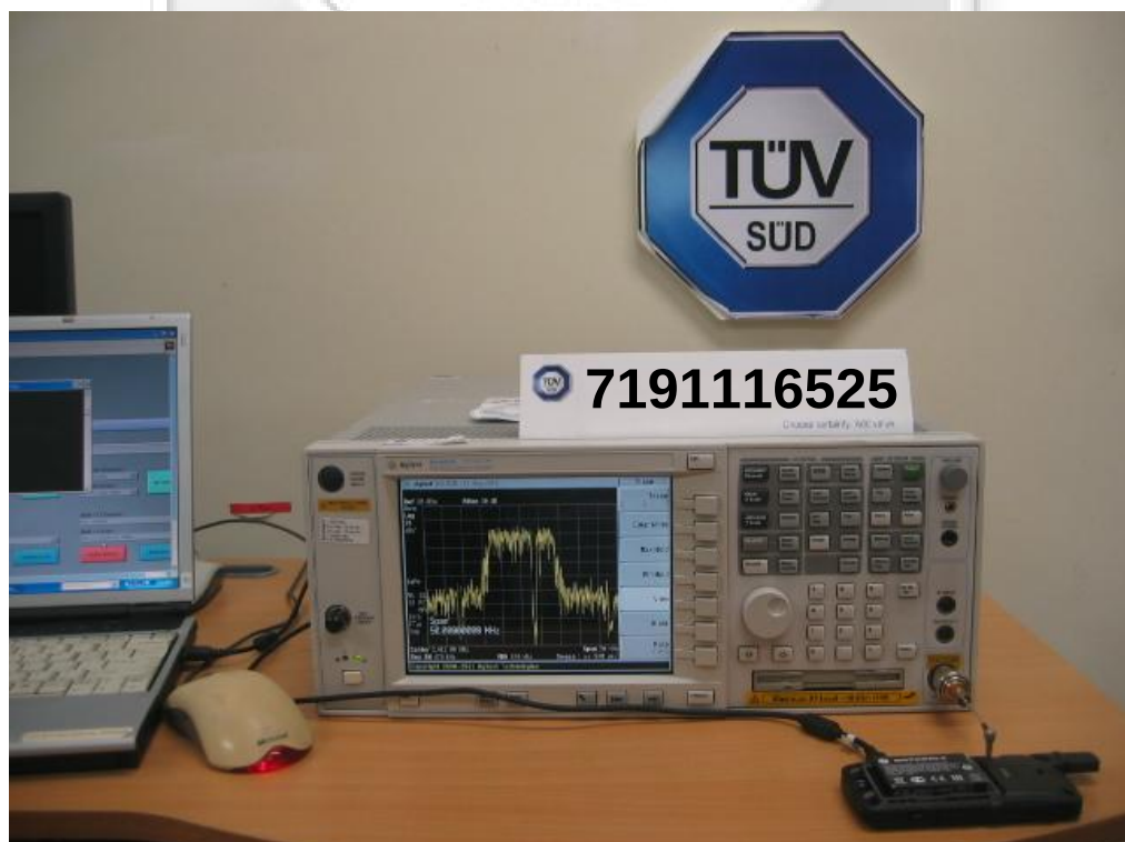
Average Frequency Dwell Time Test Setup
