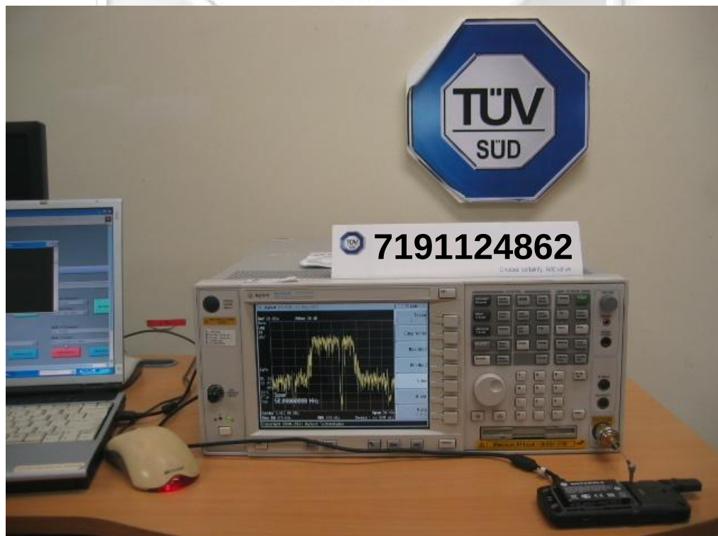
Average Frequency Dwell Time Test Setup
