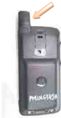
PMAF4017A (Fixed antenna pointed with arrow)
