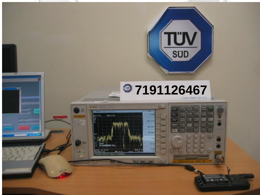
RF Conducted Spurious Emissions Test Setup
