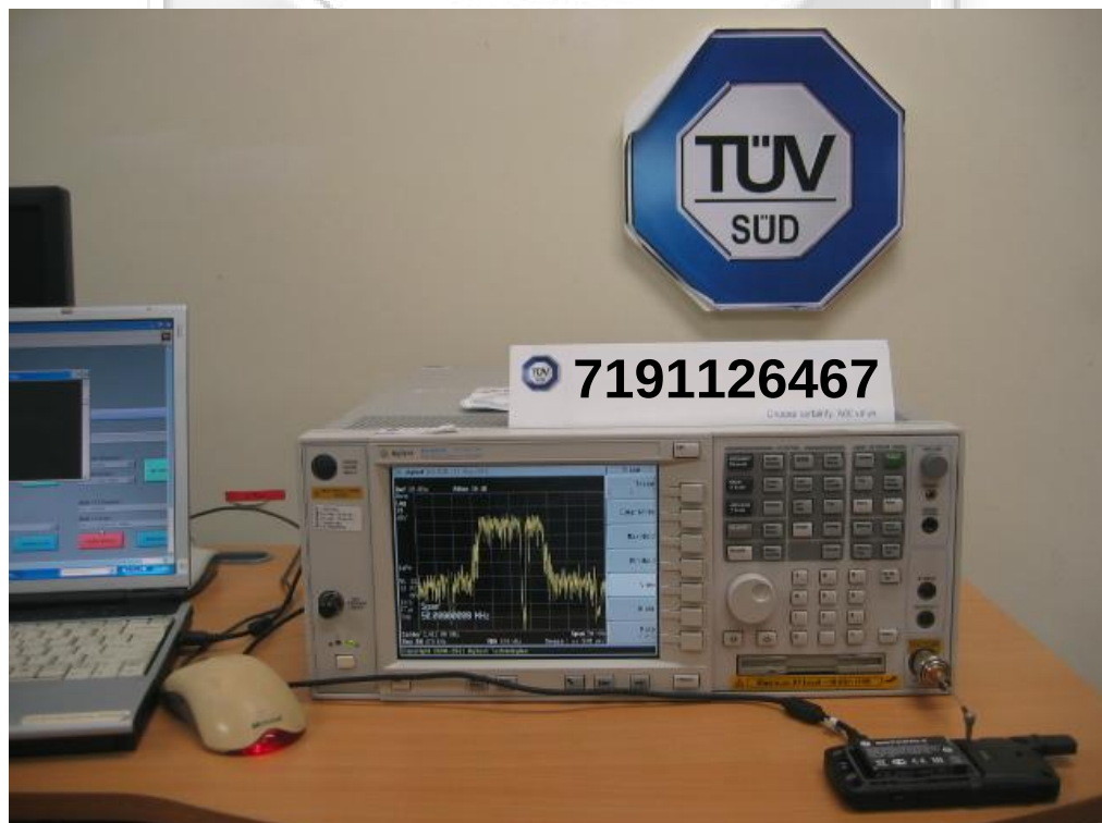
Average Frequency Dwell Time Test Setup
