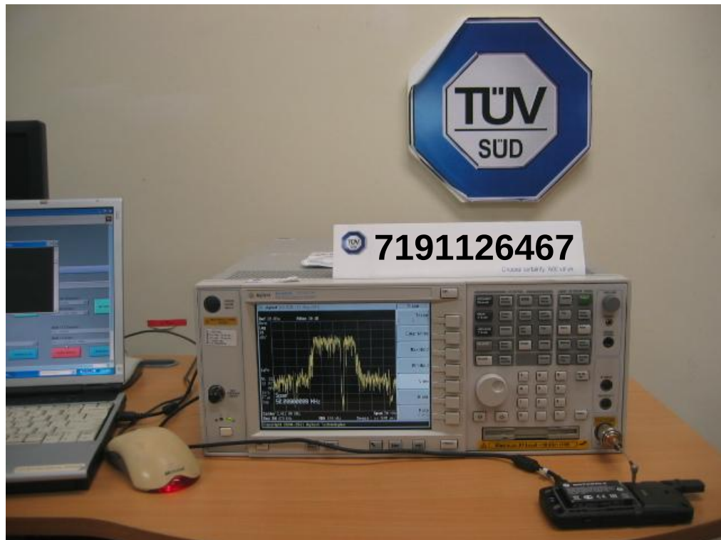
Peak Power Spectral Density Test Setup
