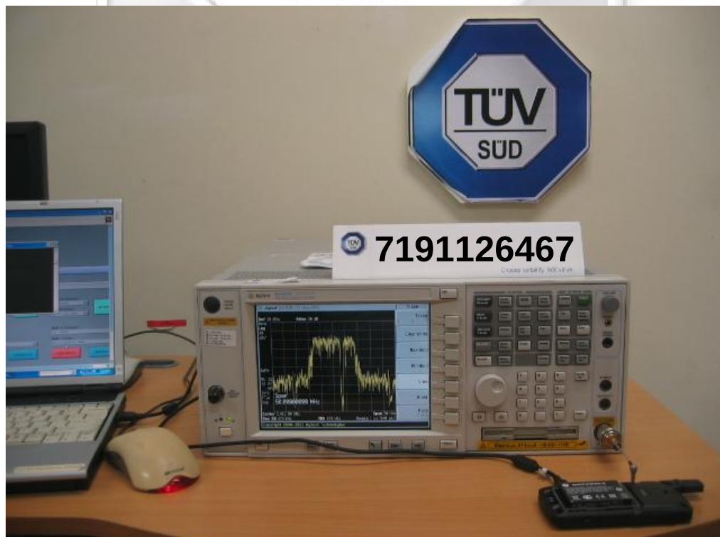
Spectrum Bandwidth (20dB Bandwidth Measurement) Test Setup
