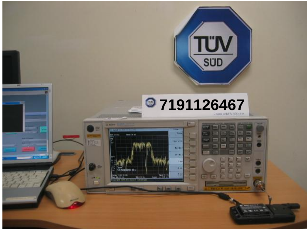
Band Edge Compliance (Conducted) Test Setup
