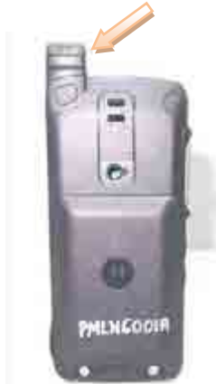
PMAF4018A (Fixed antenna pointed with arrow)
