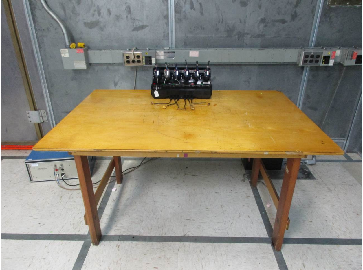
Figure 8: Power Line Conducted Emissions – Front View
