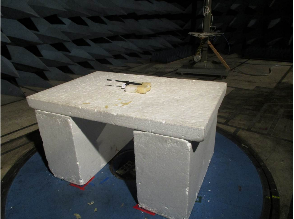
Figure 4: Radiated Emissions – Back View – 200 MHz – 1 GHz
