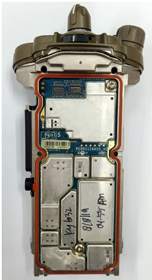
RF and Vocon boards with chassis and housing of Model 3.5 (Front side)
