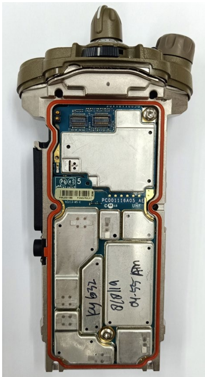
RF and Vocon boards with chassis and housing of Model 1.5 (Front side)
