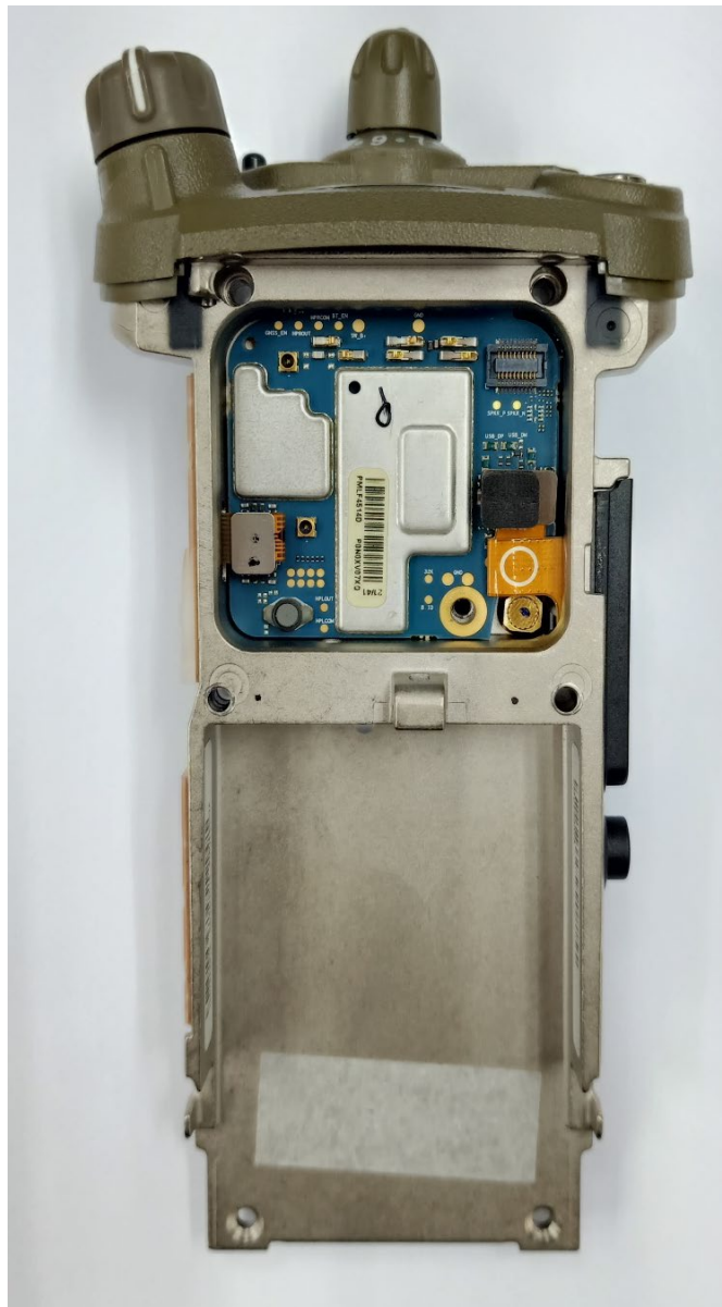
Expansion board with chassis and housing of Model 1.5 (Back side)
