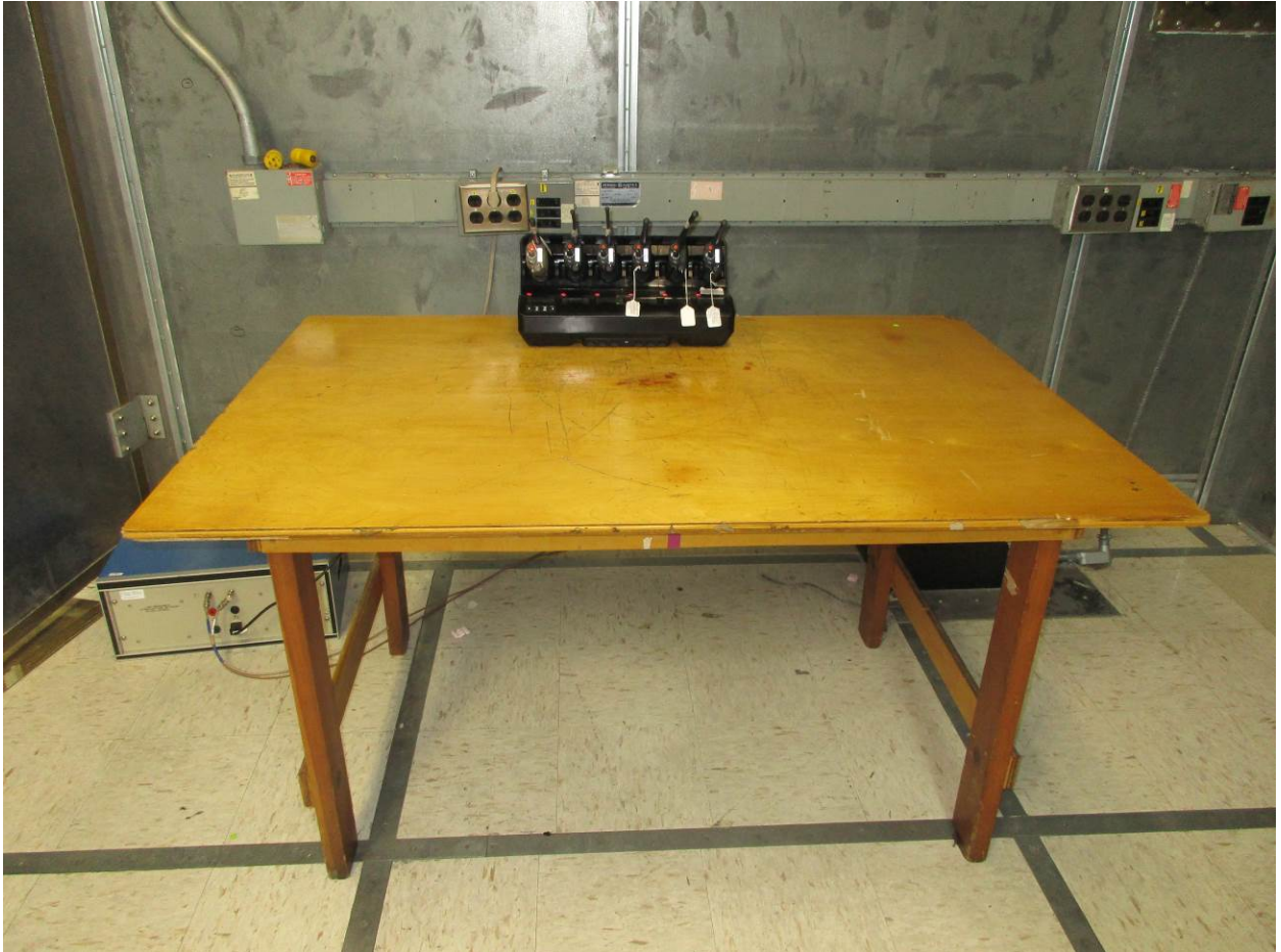
Figure 9: Power Line Conducted Emissions – Front View
