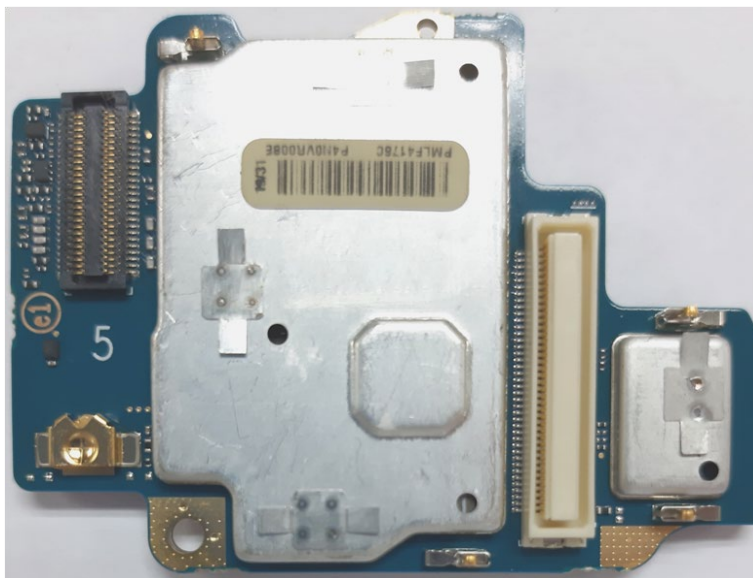
Vocon board with shields (Bottom) (APX6000/APX5000/APX6000XE/APX6000Li)
