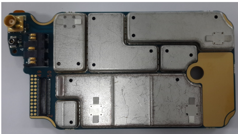
RF board with Shields (Bottom) (APX6000/APX5000/APX6000XE/APX6000Li/SRX2200)
