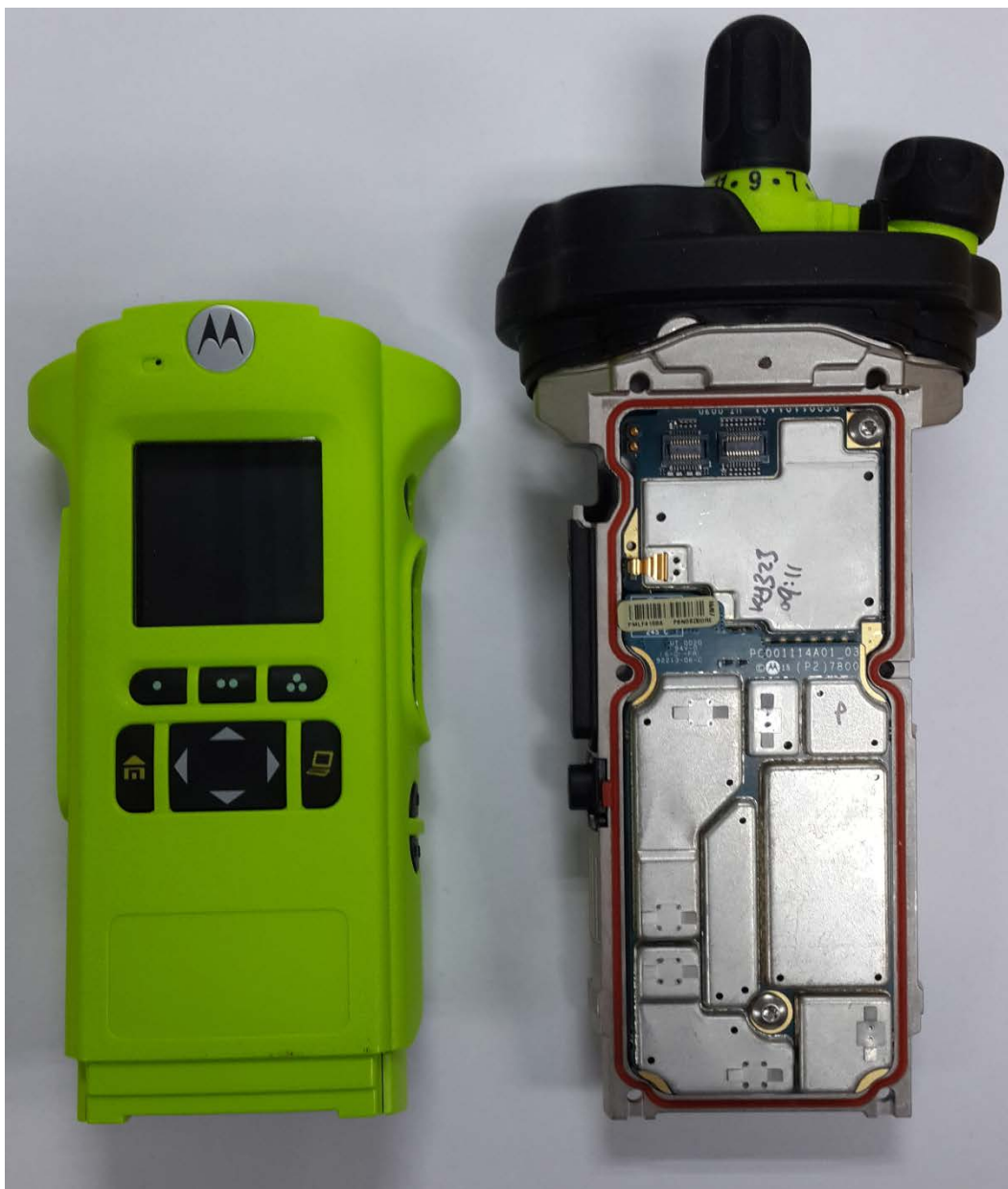
RF and Vocon boards with chassis and housing of APX6000XE Model 2.5 (Front side)
