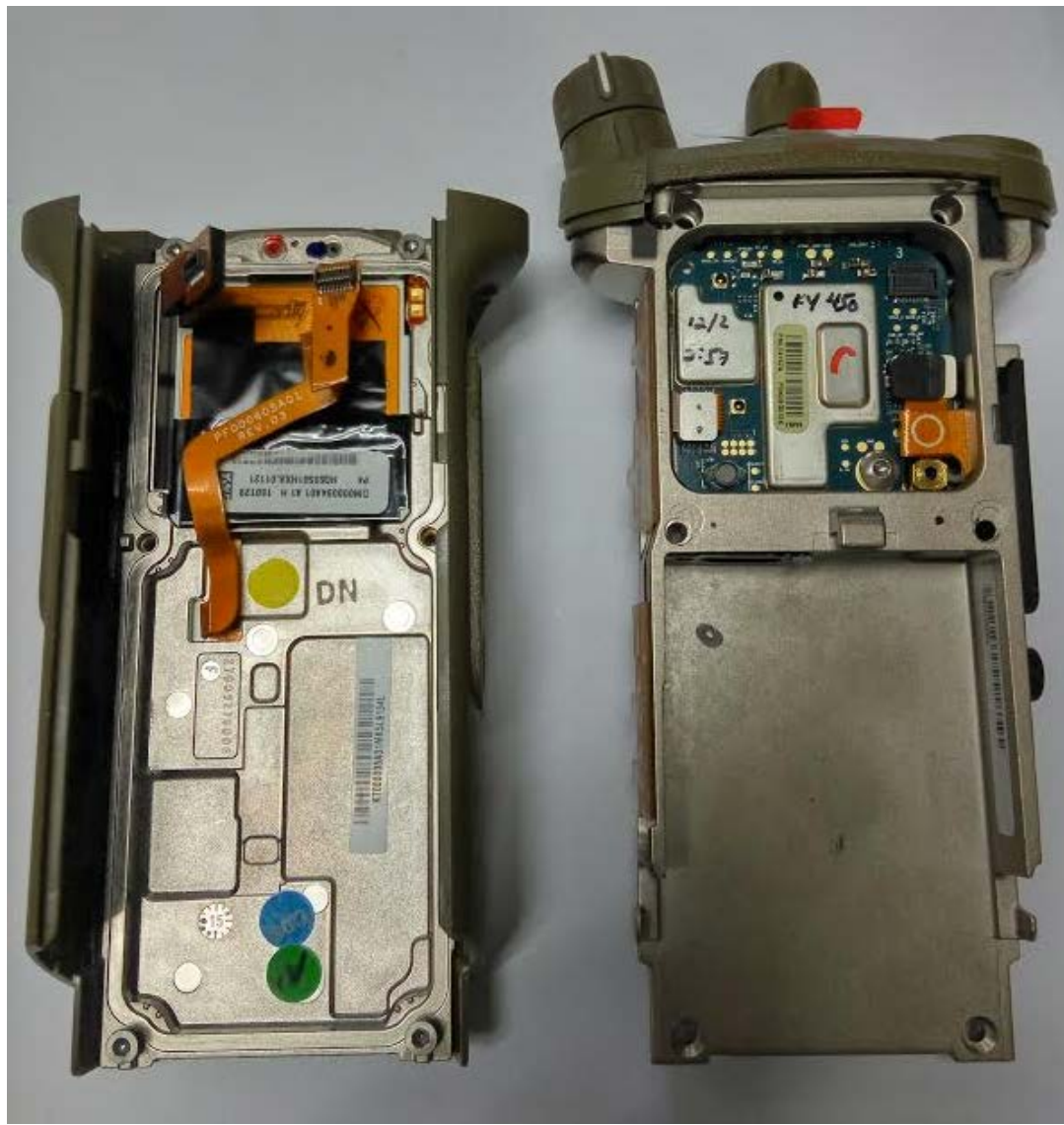
Expansion board with chassis and housing of SRX2200 Model 3.5 (Back side)
