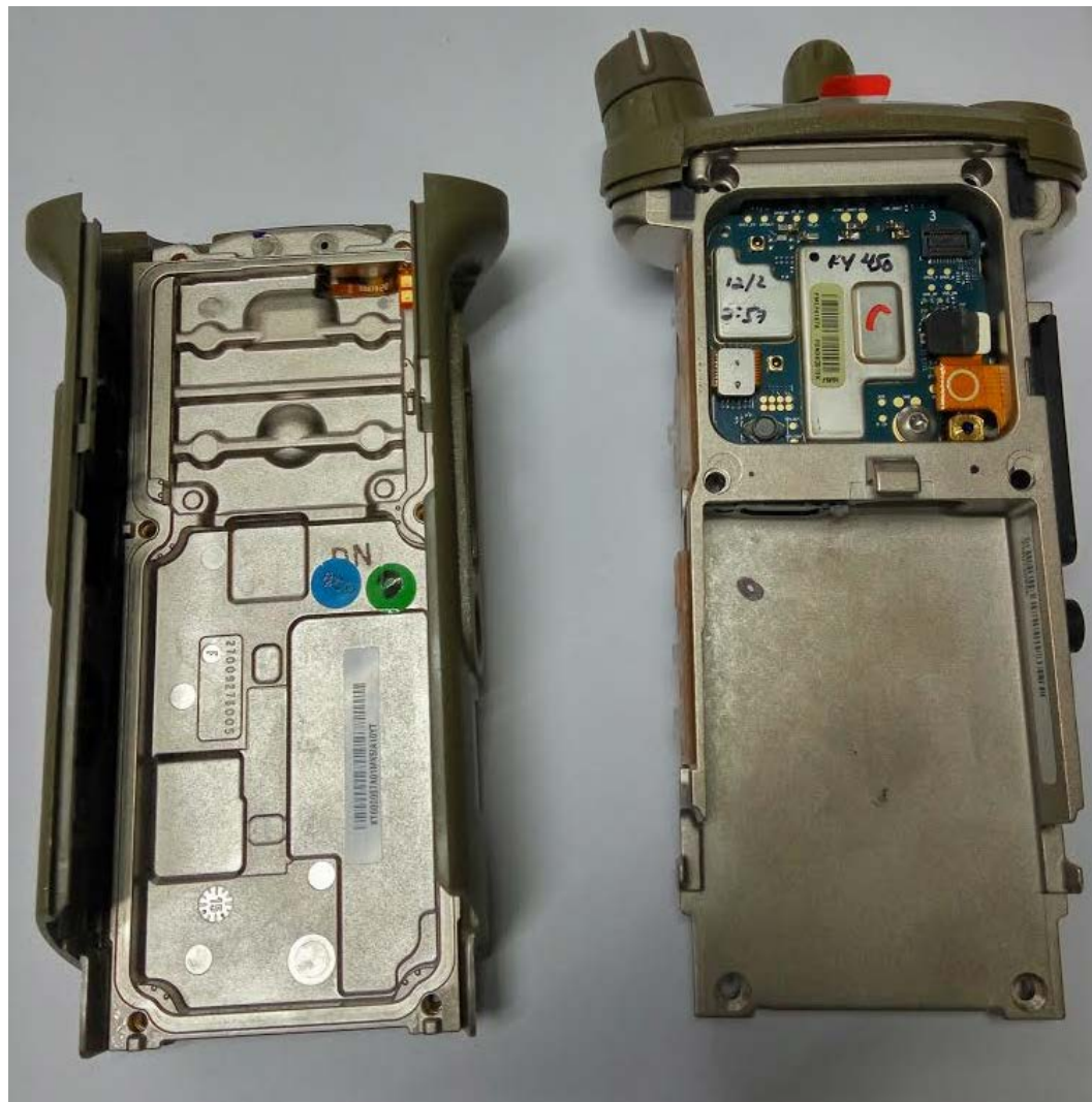
Expansion board with chassis and housing of SRX2200 Model 1.5 (Back side)
