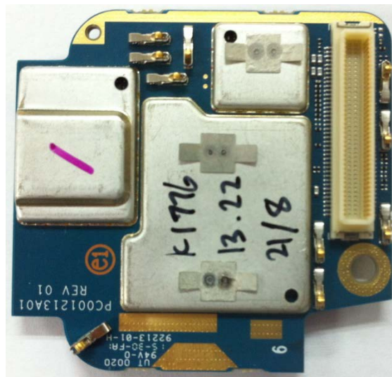
Expansion board with shields (Bottom) (APX6000/APX5000/APX6000XE/APX6000Li/SRX2200)
