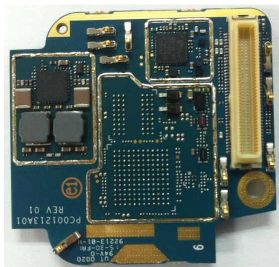
Expansion board without shields (Bottom) (APX6000/APX5000/APX6000XE/APX6000Li/SRX2200)
