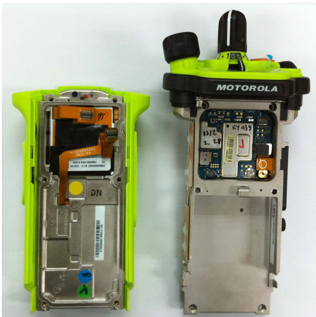
Expansion board with chassis and housing of APX6000XE Model 2.5 (Back side)
