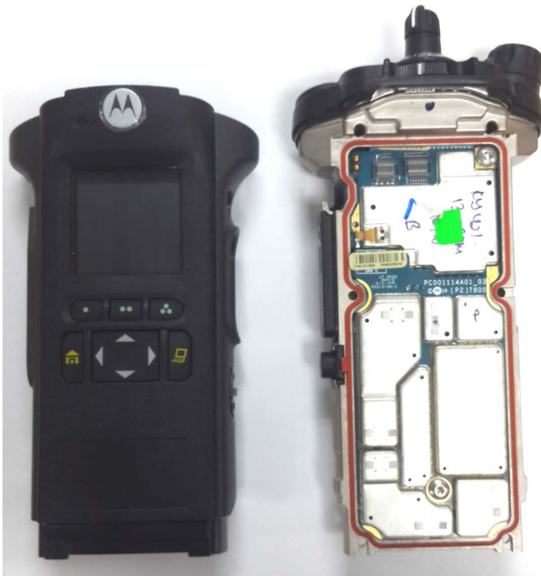
RF and Vocon boards with chassis and housing of APX6000/APX6000Li/APX5000 Model 2.5 (Front side)
