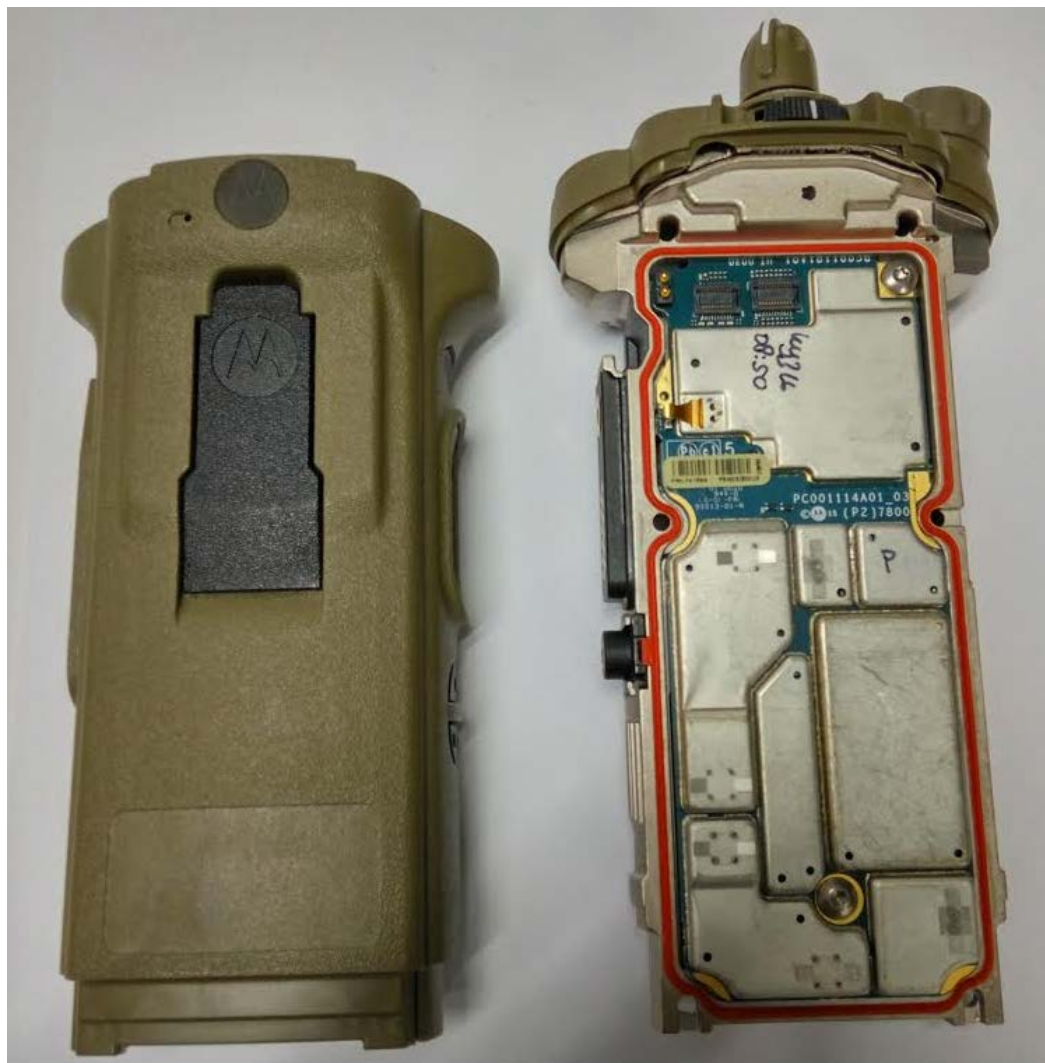
RF and Vocon boards with chassis and housing of SRX2200 Model 1.5 (Front side)
