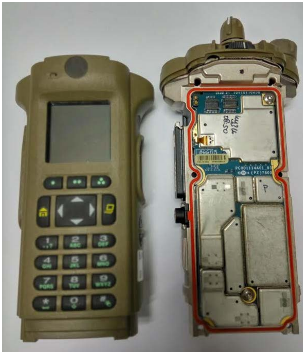
RF and Vocon boards with chassis and housing of SRX2200 Model 3.5 (Front side)
