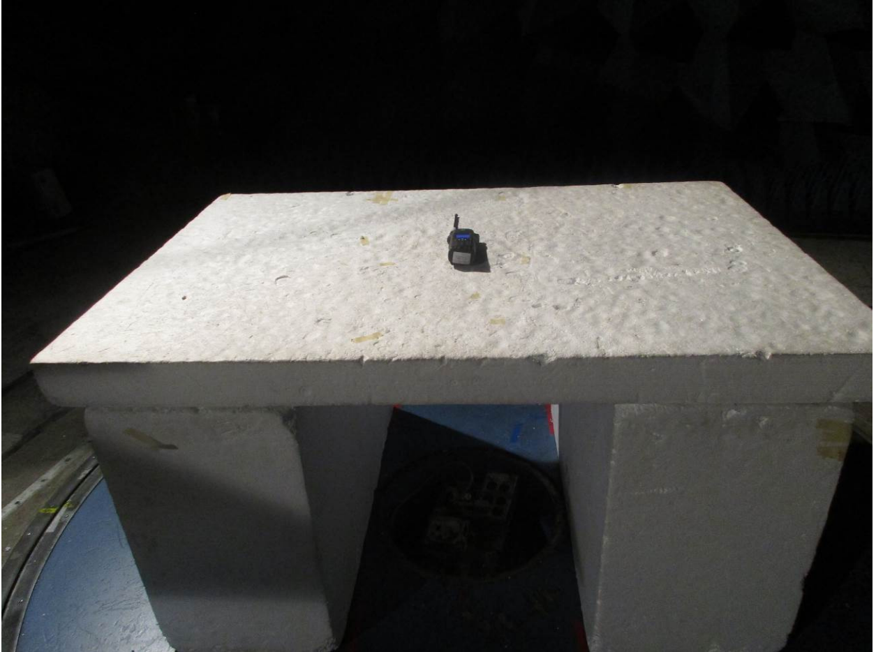
Figure 3: Radiated Emissions – Front View – Below 1 GHz
